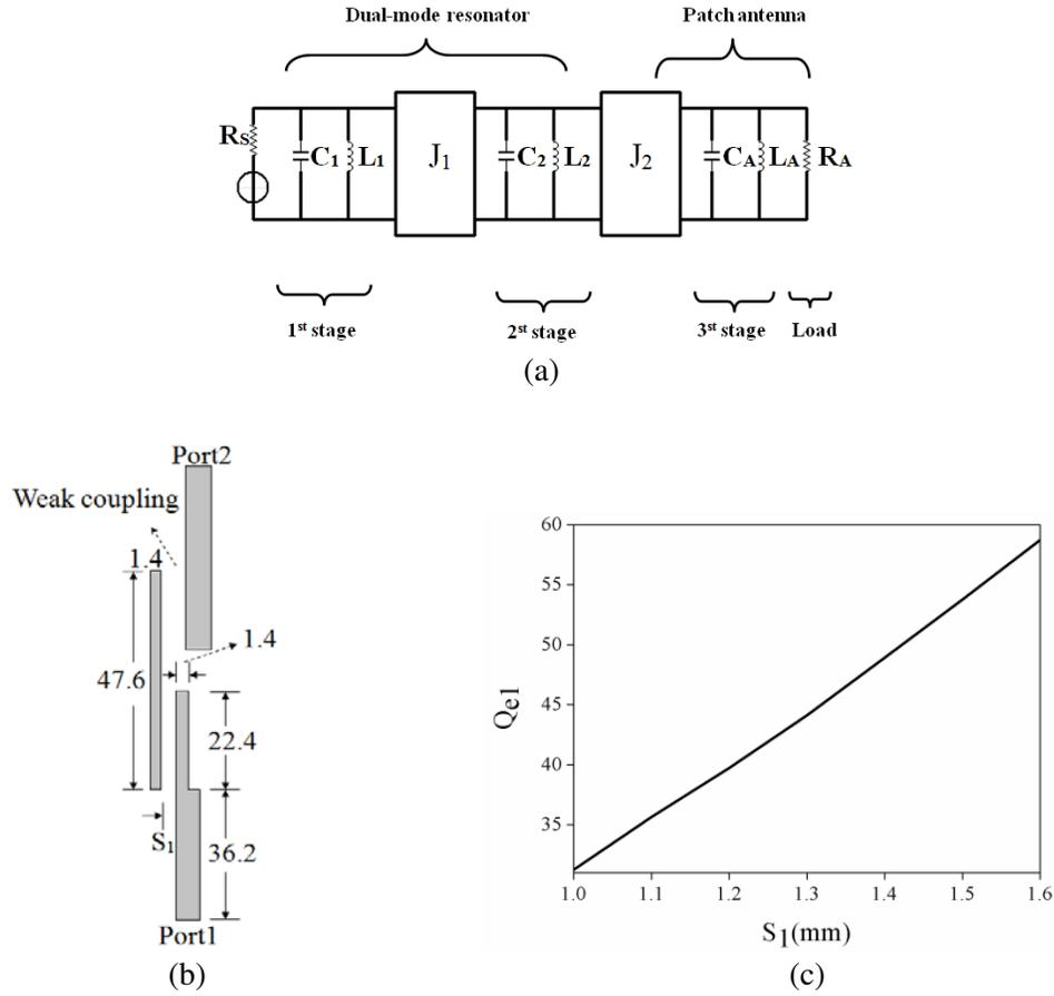
**Figure 1.** (a) Equivalent circuit of the proposed antenna; (b) The arrangement for the extraction of the input/output external quality factor (unit: mm); (c) The curve of the external quality factor  $Q_{e1}$  with respect to gap  $S_1$ .
