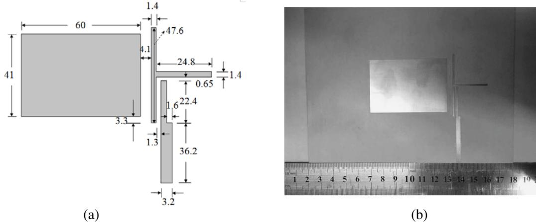
**Figure 5.** (a) The layout of proposed filtering antenna (unite: mm); (b) The photograph of the fabricated antenna.
