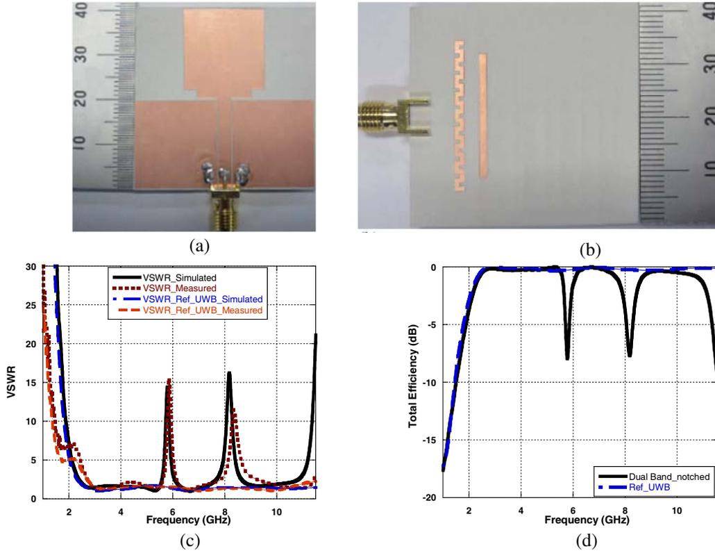
**Figure 4.** Photographs of the proposed fabricated dual band-notched antenna, VSWR, and efficiencies: (a) Top layer. (b) Bottom layer. (c) Measured and simulated VSWR. (d) Simulated total efficiencies.
