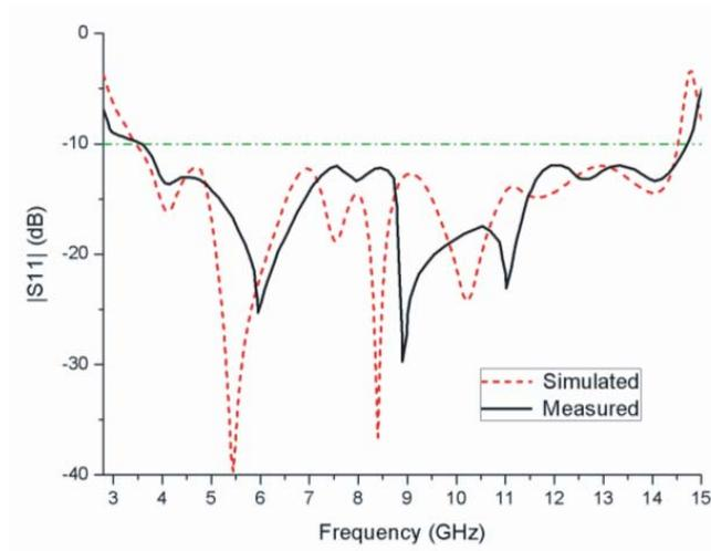
Figure 6. Measured and simulated  $|S_{11}|$  against frequency.
