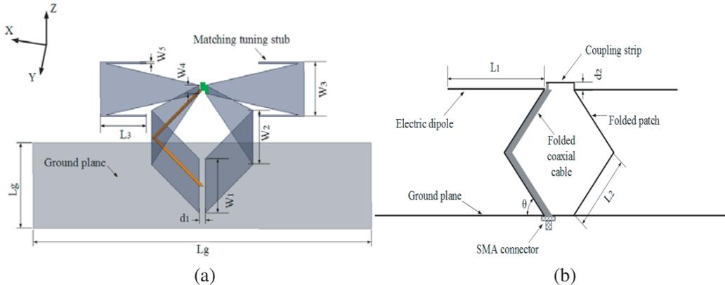
**Figure 1.** Geometry of the electrical-magnetic composite antenna: (a) 3D view; (b) Side view.
