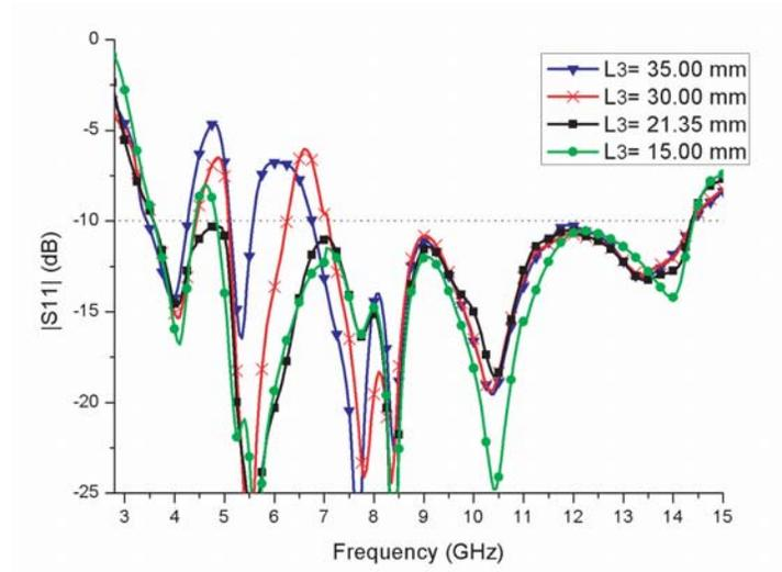
Figure 4. Effects of various tuning stubs' length  $L_3$ .
