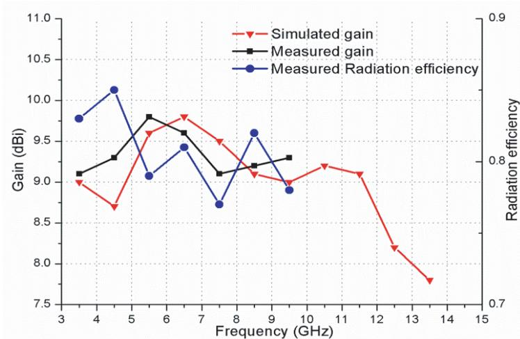
**Figure 8.** Gains and radiation efficiency of the proposed antenna.
