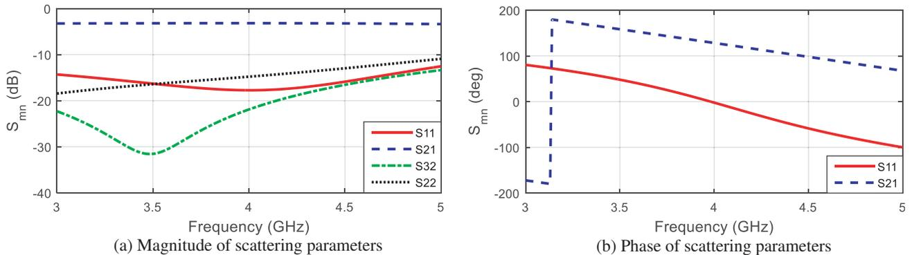
Figure 5. Scattering parameters of the power divider element.
