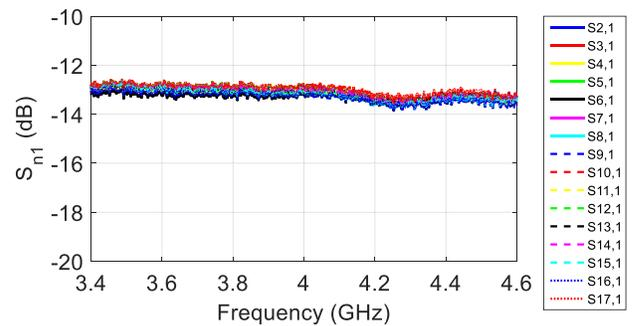
**Figure 9.** Magnitude of measured transmission coefficients.
