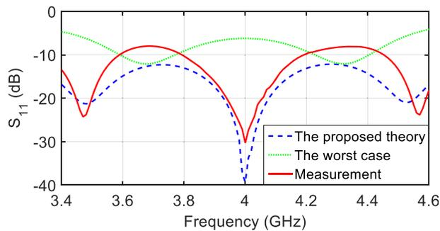
**Figure 8.** Calculated and measured reflection coefficient of 4-stage power divider designed with perfect match at 4 GHz, and calculated reflection coefficient of 4-stage power with worst return loss at 4 GHz.
