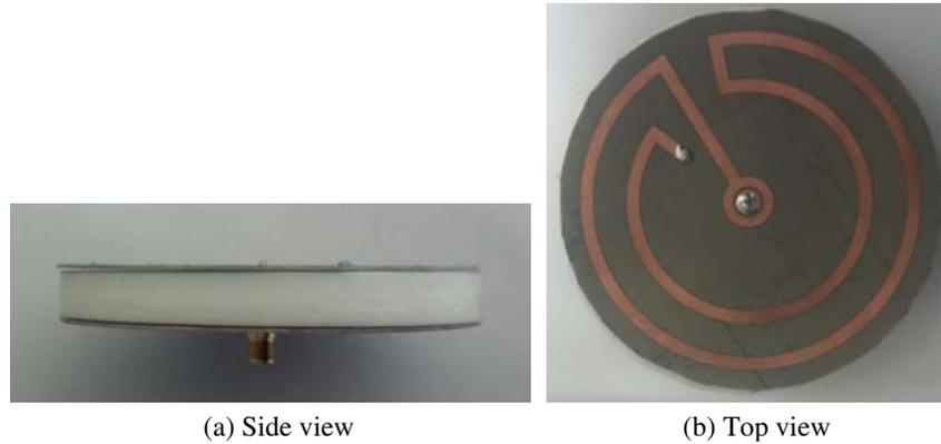
**Figure 8.** Photograph of the fabricated antenna.
