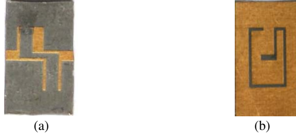
Figure 4. Photographs of the implemented HPF. (a) Top microstrip, and (b) bottom improved U-shaped slot resonator embedded with L-shaped slot.
