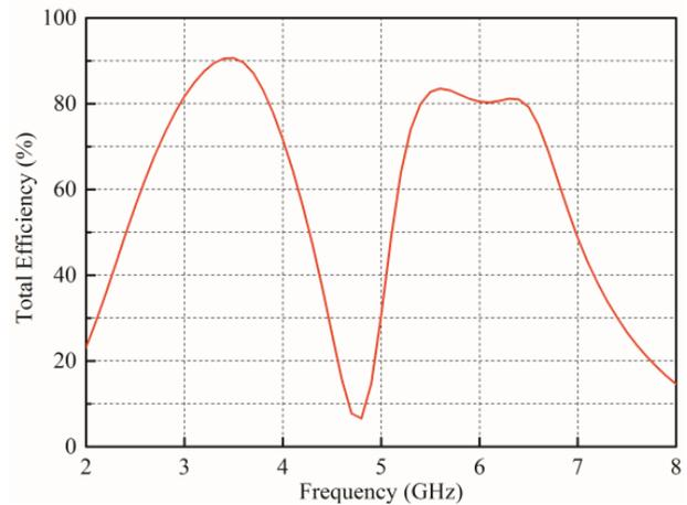
**Figure 8.** Simulated total efficiency of the proposed antenna.
