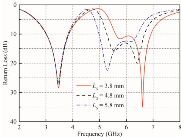
**Figure 3.** Simulated return loss for the proposed antenna with varying length  $L_S$  of the slot stubs
