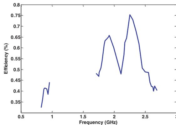
Figure 9. Measured radiation efficiency for the fabricated antenna.
