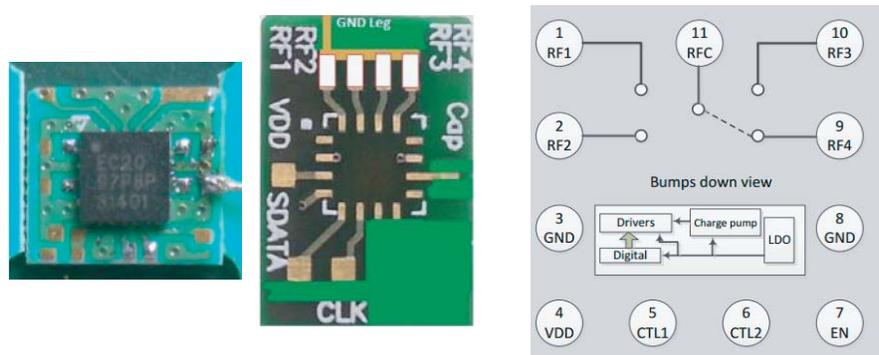
Figure 3. Pictures and functional schematic of RF switches.
