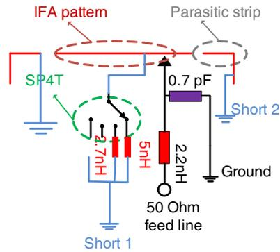
Figure 2. The schematic diagram of the proposed antenna.
