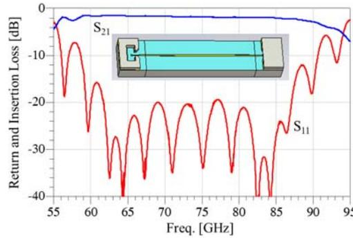
**Figure 5.** Simulated results of the MSL-to-WR12 transition in back-to-back structure [The inset is a 3 dimensional structure for simulation of the transition in back-to-back type and the closure is open in the left transition].
