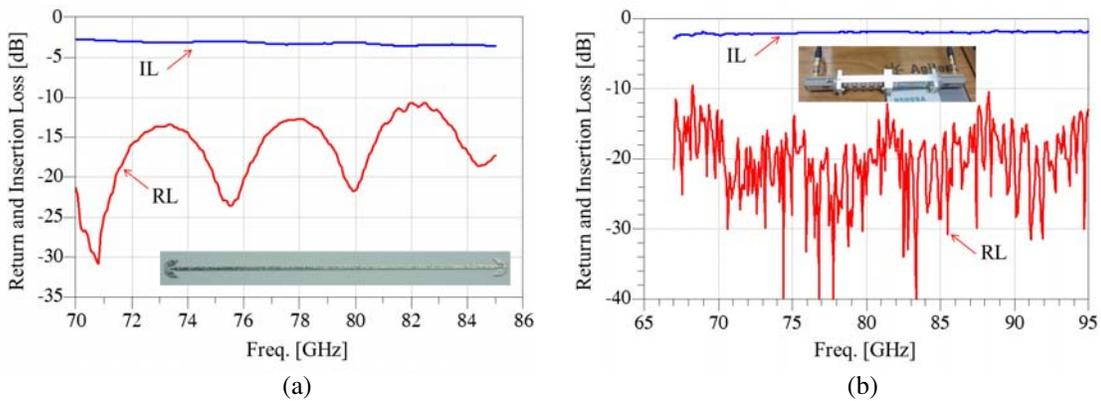
**Figure 7.** Measured return and insertion loss of a (a) MSL and (b) connections of a cable-to-WG adapter and WG transition [Inset of (a) and (b) are the fabricated 20.6 mm-long MSL and connections of cable-to-WG adapters and WR10-to-WR12 transitions, respectively].
