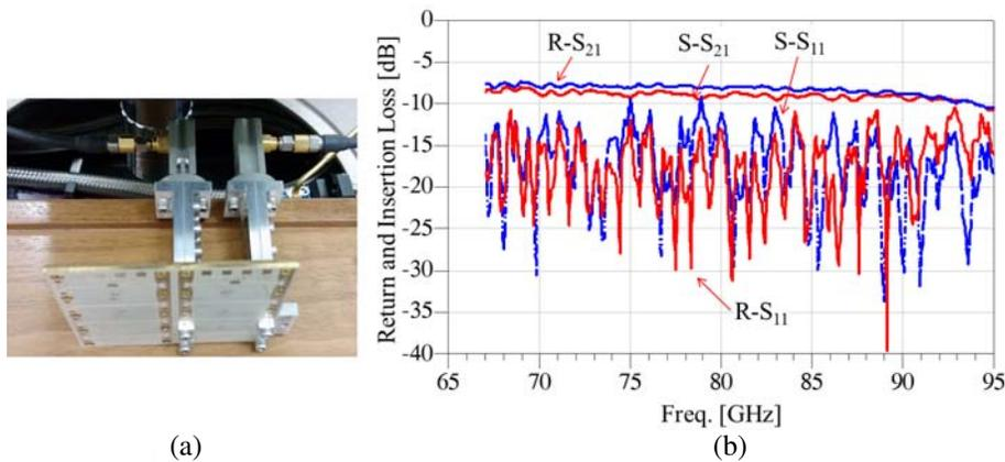
**Figure 8.** A test set-up of the fabricated MSL-to-WR12 WG transitions using the R-probe and eGND planes in (a) back-to-back type and (b) its measured results [R- and S-: Transition with R-probe and S-probe, respectively].
