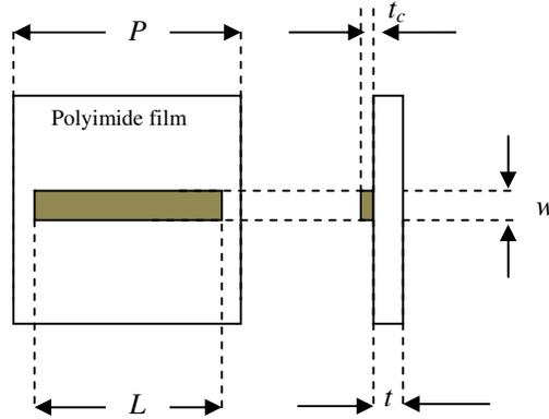
**Figure 1.** The unit cell of the dipole FSS.
