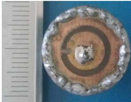
**Figure 4.** Photo of the fabricated CP antenna.
