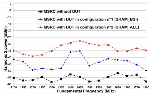
**Figure 7.** Measurement of second-order harmonic frequency levels.
