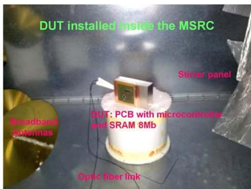
**Figure 6.** DUT located inside MSRC.
