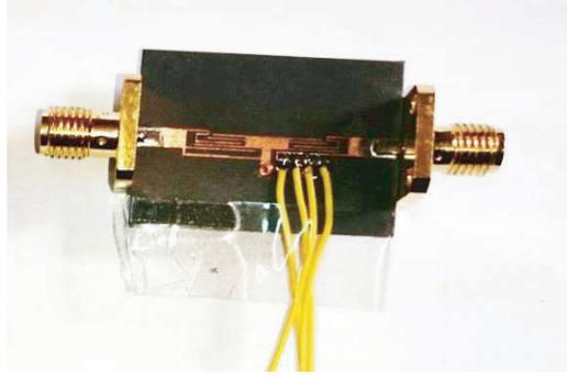
**Figure 3.** A photo for the fabricated filter.
