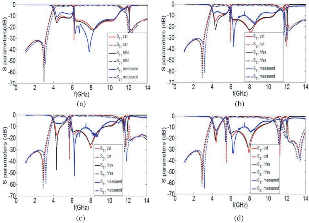
**Figure 4.** The simulated and measured  $S_{11}$  and  $S_{21}$  for different  $L_6$  lengths. (a)  $L_6 = 2.0$  mm, (b)  $L_6 = 3.1$  mm, (c)  $L_6 = 4.2$  mm, (d)  $L_6 = 5.3$  mm.
