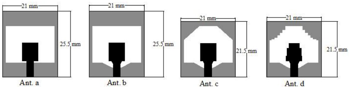
**Figure 2.** Miniaturized design process of the proposed antenna.
