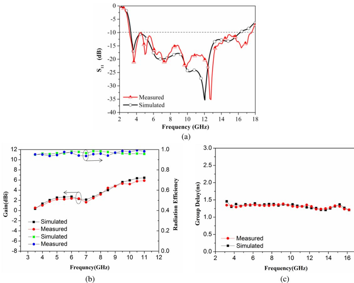
**Figure 5.** (a) Simulated and measured return loss curves of the fabricated antenna; (b) Simulated and measured total gains and radiation efficiencies of the proposed antenna; (c) Simulated and measured group delays for the proposed UWB antenna.
