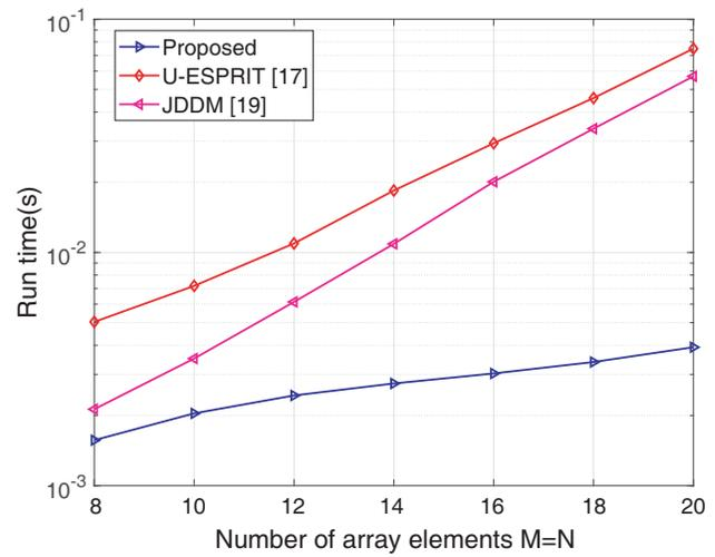
Figure 6. Run time versus the elements number.
