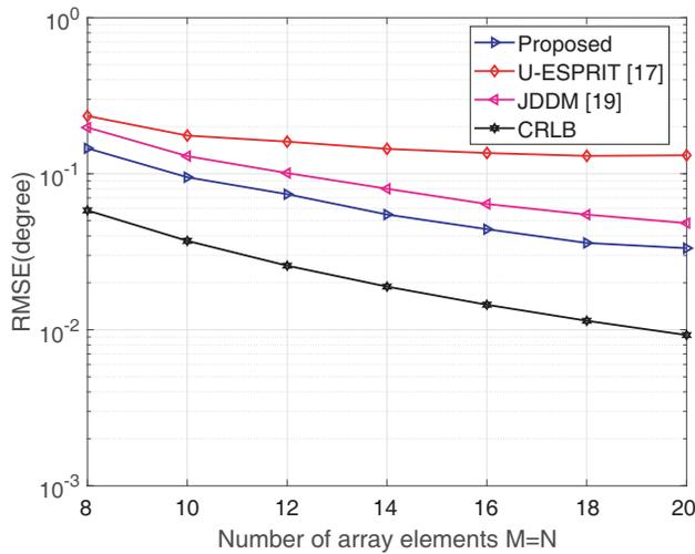
Figure 5. RMSE versus the elements number.
