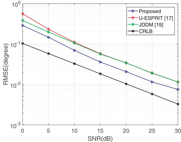
**Figure 3.** RMSE versus SNR with  $L = 50$ .
