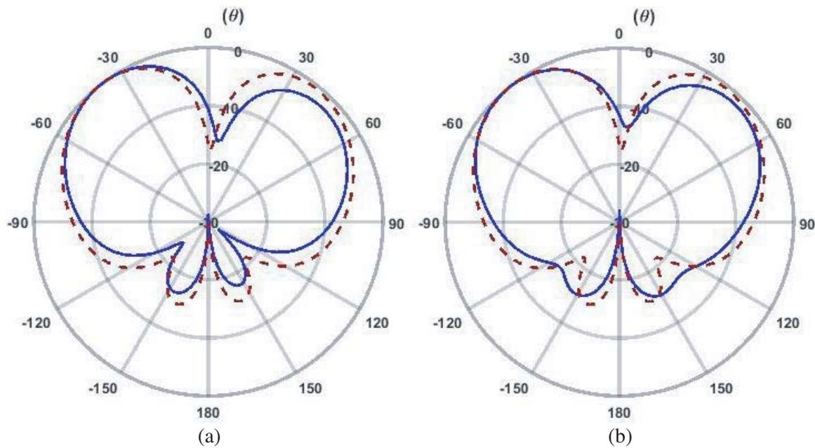
**Figure 6.** Measured and simulated radiation patterns of the fabricated antenna at 3 GHz, when  $L = 13$  mm and  $\alpha = 4.2^\circ$ ; (a)  $E$ -plane, (b)  $H$ -plane; — Measured pattern, ---- Simulated pattern.
