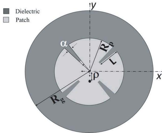
**Figure 2.** Geometry of the proposed slit-loaded  $TM_{21}$  circular patch antenna with  $R_p = 19.25$  mm,  $R_g = 60$  mm,  $\rho = 4.2$  mm,  $\epsilon_r = 2.2$ , and substrate thickness of 1.6 mm.
