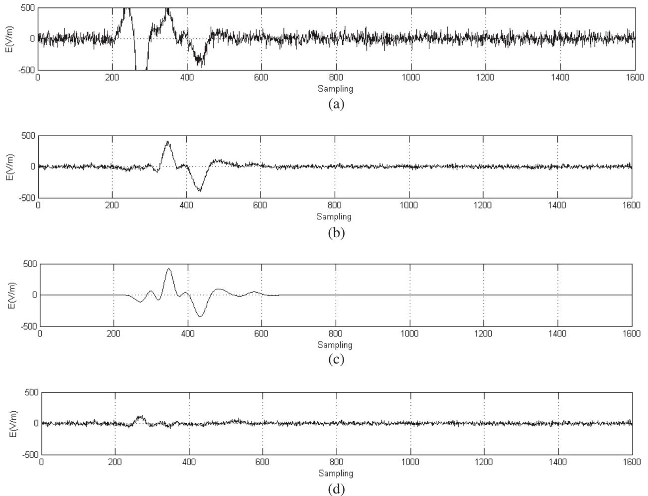
**Figure 2.** Results of enhanced GPR target signal using proposed method under rough surface with  $\text{SNR} = 0$  dB, landmine depth = 0.5 cm: (a) original signal contaminated with ground clutter and background noise  $\text{SNR} = 0$  dB, (b) enhanced signal using proposed method, (c) reference signal (landmine only), (d) residual signal produced by subtract signal (c) to (b).
