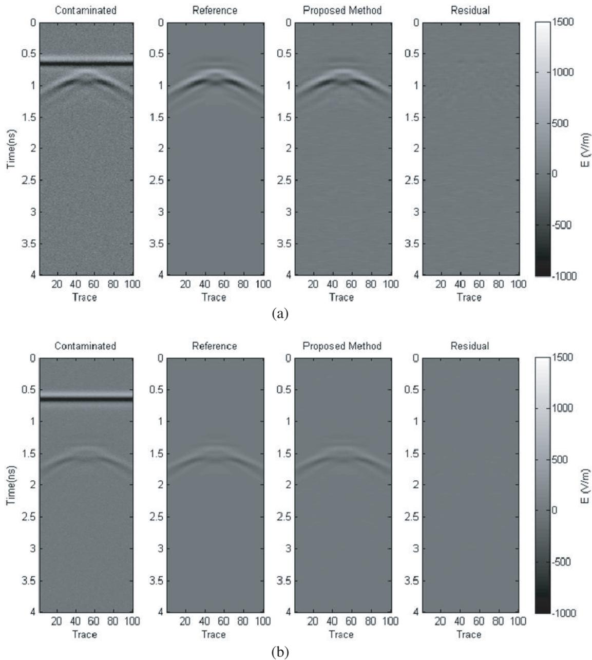
**Figure 3.** Results of enhanced GPR target signal using proposed method under flat surface with  $\text{SNR} = 0\text{ dB}$  and its comparison with the reference signal (landmine only): (a) landmine depth is 0.5 cm, (b) landmine depth is 5 cm.
