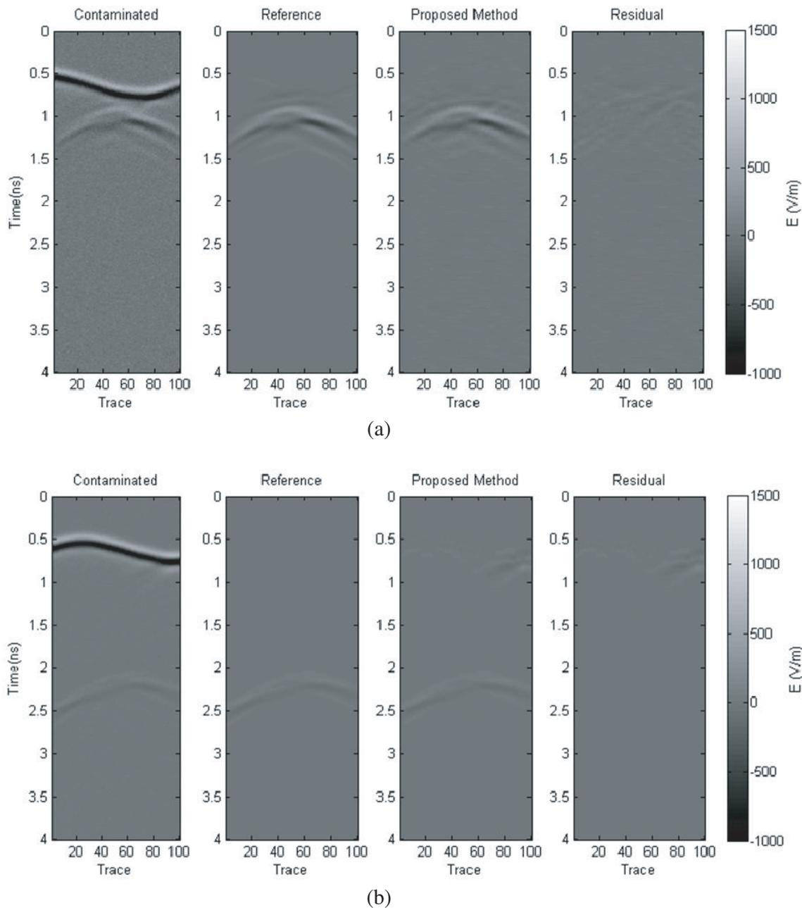
**Figure 4.** Then please change the figure and caption syntax as below, Results of enhanced GPR target signal using proposed method under rough surface with  $\text{SNR} = 0\text{ dB}$  and its comparison with the reference signal (landmine only): (a) landmine depth is 2 cm, (b) landmine depth is 10 cm.
