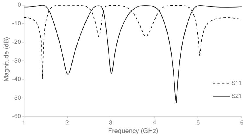
**Figure 6.** Simulation results of the second order BSF.
