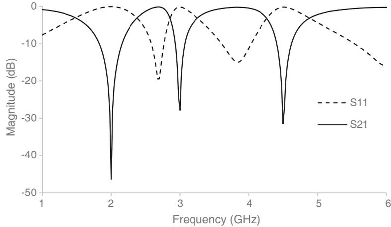
**Figure 4.** Simulation results of the tuned first order triband BSF.
