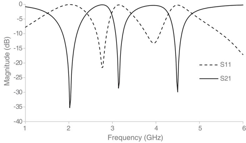
**Figure 3.** Simulation results of the first order triband BSF.
