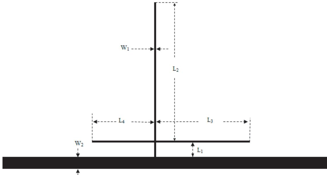
**Figure 2.** Layout of the first order triband BSF.
