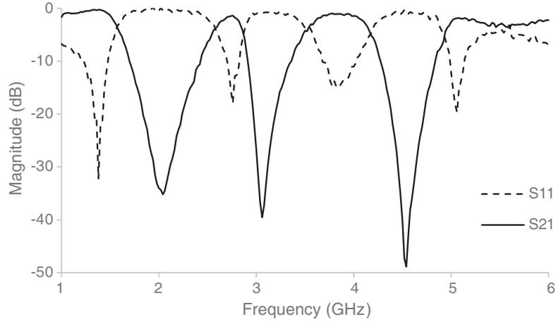
**Figure 8.** 2nd order triband BSF measurement results.
