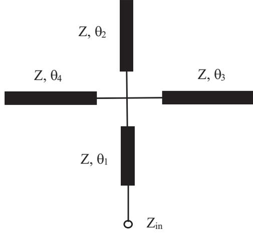
**Figure 1.** The structure of the proposed asymmetrical cross-shaped resonator.
