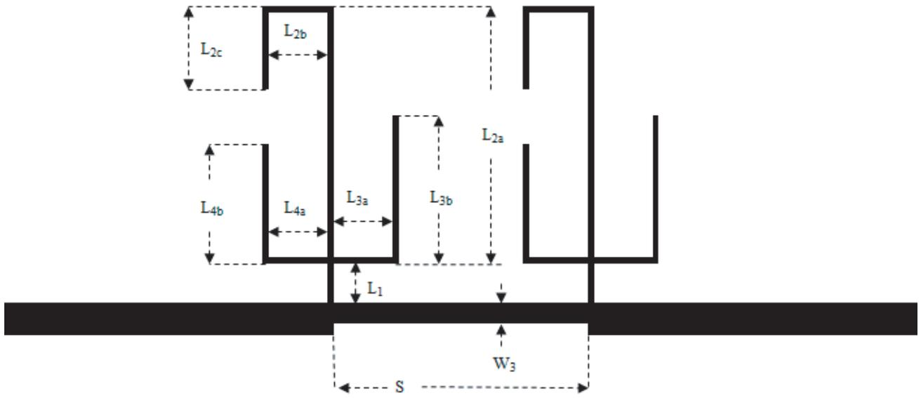
**Figure 5.** Layout of the tuned second order triband BSF.
