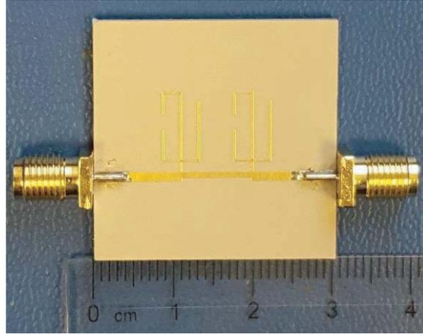
**Figure 7.** Fabricated 2nd order triband BSF.
