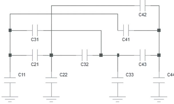
**Figure 1.** Capacitive coupling diagram of differential line.
