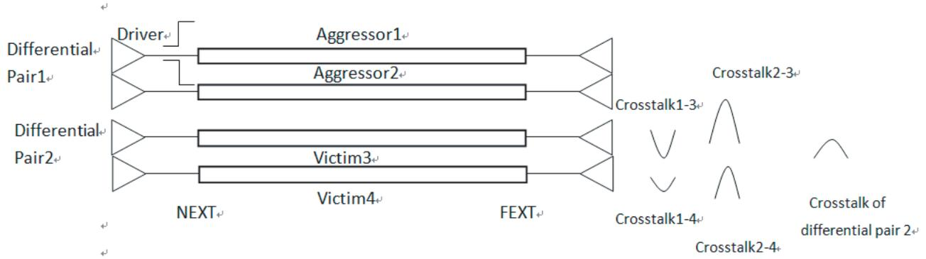
Figure 3. The FEXT diagram between differential line pairs.
