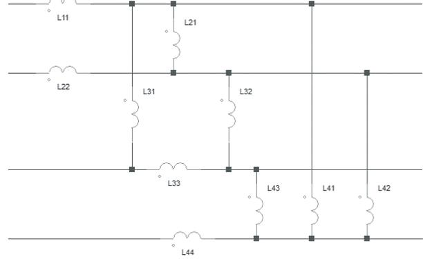
**Figure 2.** Inductive coupling diagram of differential line.
