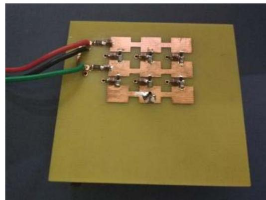
**Figure 6.** Pixel antenna with PIN diodes and bias circuit.
