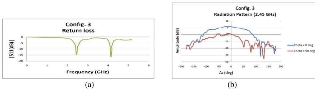
**Figure 10.** Measurement results of Configuration 3: When all PIN diodes are ON. (a)  $S_{11}$  parameter for Config. 3 when  $V_1 = 5$  V and  $V_2 = 5$  V. (b) Radiation pattern for Config. 3 for theta = 0 deg and 90 deg.
