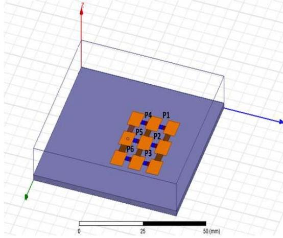
**Figure 4.** Pixel antenna with PIN diodes in HFSS.
