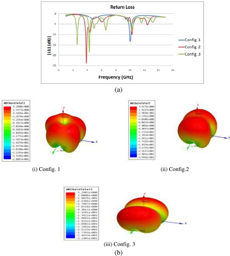
**Figure 5.** (a)  $S_{11}$  parameter for the different configurations: Config. 1 when all PIN diodes are OFF; Config. 2 When PIN diodes P4, P5, P6 ON; Config. 3 When all PIN diodes ON. (b) Radiation pattern for all the three configurations.
