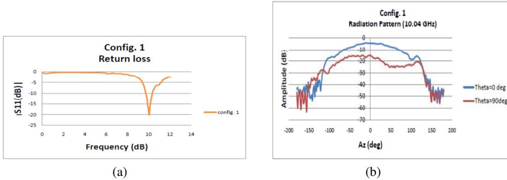
**Figure 8.** Measurement results of Configuration 1: when all PIN diodes are OFF. (a)  $S_{11}$  parameter for config. 1 when  $V_1 = 0$  V and  $V_2 = 0$  V. (b) Radiation pattern for Config. 1 for theta = 0 deg and 90 deg.
