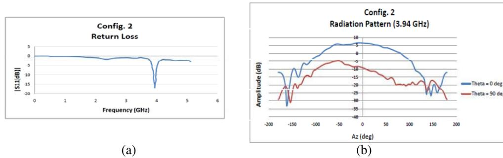
**Figure 9.** Measurement results of Configuration 2: When one row of PIN diodes (P4, P5 and P6) are ON. (a)  $S_{11}$  parameter for Config. 2 when  $V_1 = 0$  V and  $V_2 = 5$  V. (b) Radiation pattern for Config. 2 for theta = 0 deg and 90 deg.
