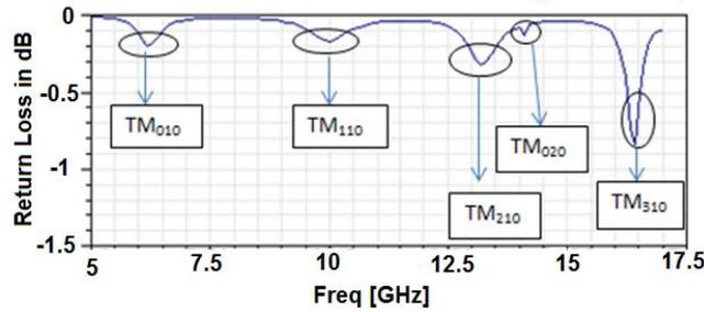
**Figure 2.** The simulated return loss of FMSIW cavity.
