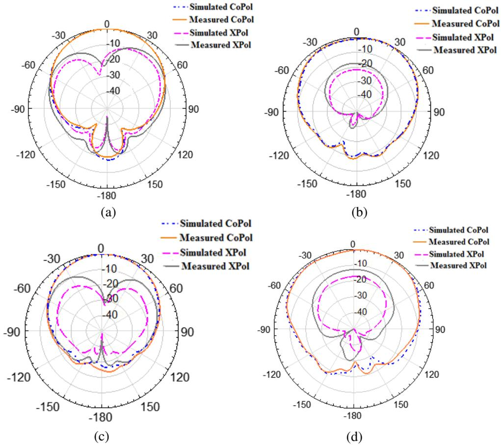
**Figure 11.** Simulated and measured (a)  $E$ -Plane ( $\phi = 90^\circ$ ) pattern at 8.5 GHz (b)  $H$ -Plane ( $\phi = 0^\circ$ ) pattern at 8.5 GHz (c)  $E$ -Plane ( $\phi = 90^\circ$ ) Patternn at 10.6 GHz (d)  $H$ -Plane ( $\phi = 0^\circ$ ) pattern at 10.6 GHz.
