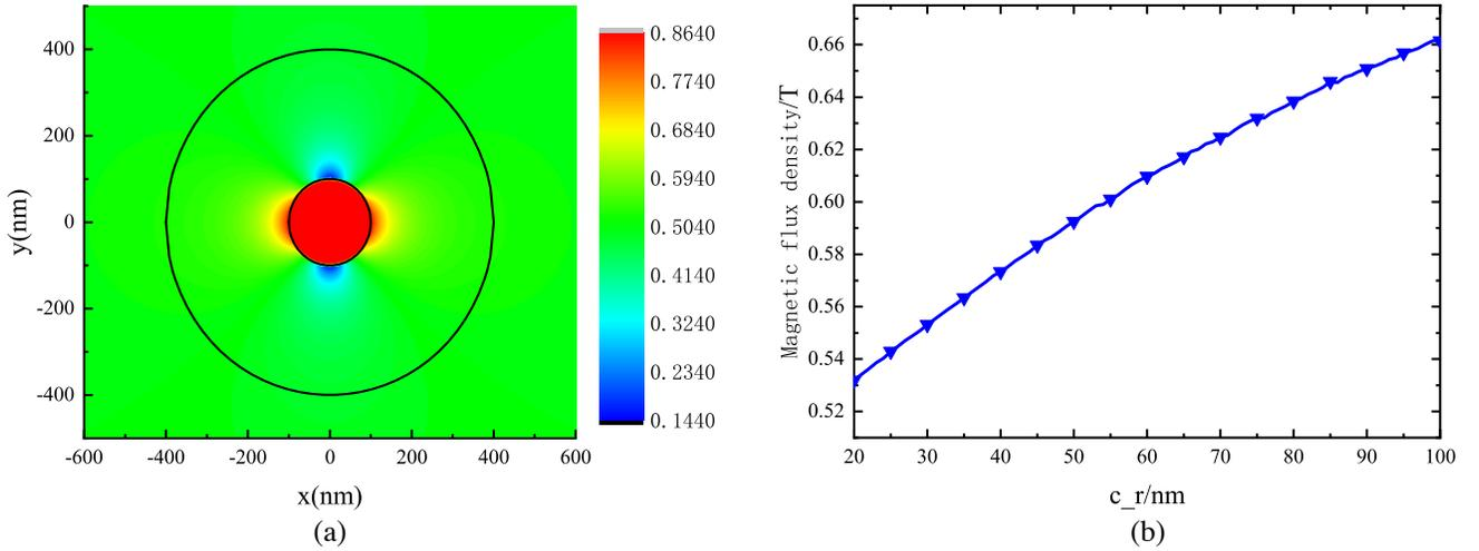
**Figure 5.** The influence of magnetic nanoparticle radius on magnetic flux density. (a)  $r = 100$  nm magnetic flux density distribution plan. (b) The relationship between magnetic flux density and radius.
