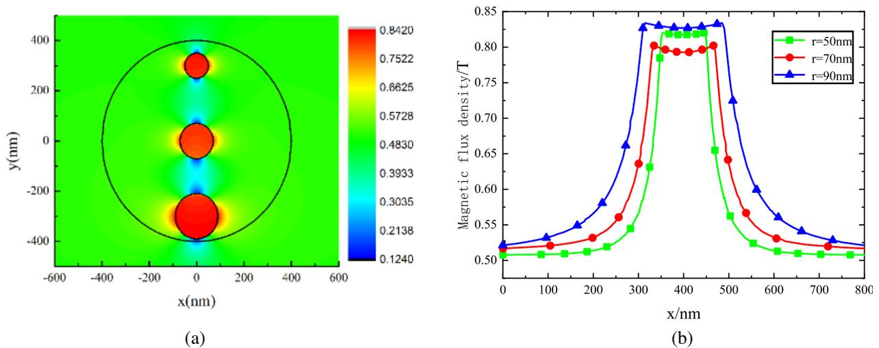
**Figure 3.** Flux density distribution of MNPs with different radii. (a) Flux density two-dimensional distribution. (b) Flux density one-dimensional curve.
