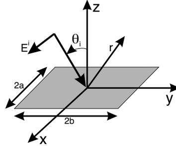
**Figure 1.** Thin conducting plate illuminated by an obliquely incident plane wave.
