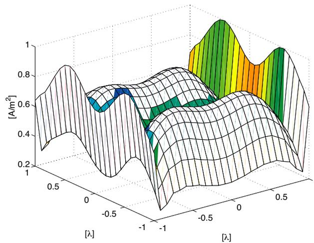
**Figure 5.** 3D plot of the dominant current  $J_x$  on a  $2\lambda \times 2\lambda$  metal plate.
