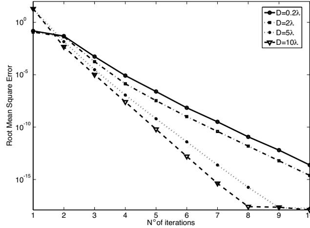
**Figure 3.** Root mean square error for different values of the plate side  $D$  (local-edge solution as initial guess for the current).
