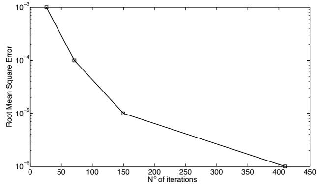
**Figure 4.** Convergence rate of the Conjugate Gradient method for a square plate of side  $D = \lambda$  (from [29]).
