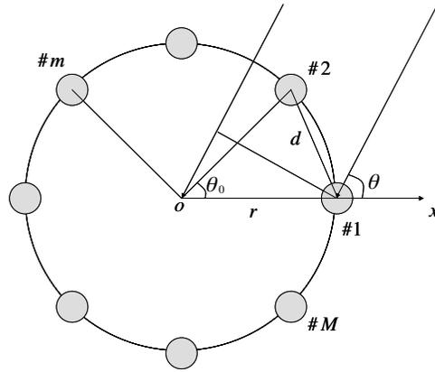
**Figure 1.** Geometry of the UCA with  $M$  elements.
