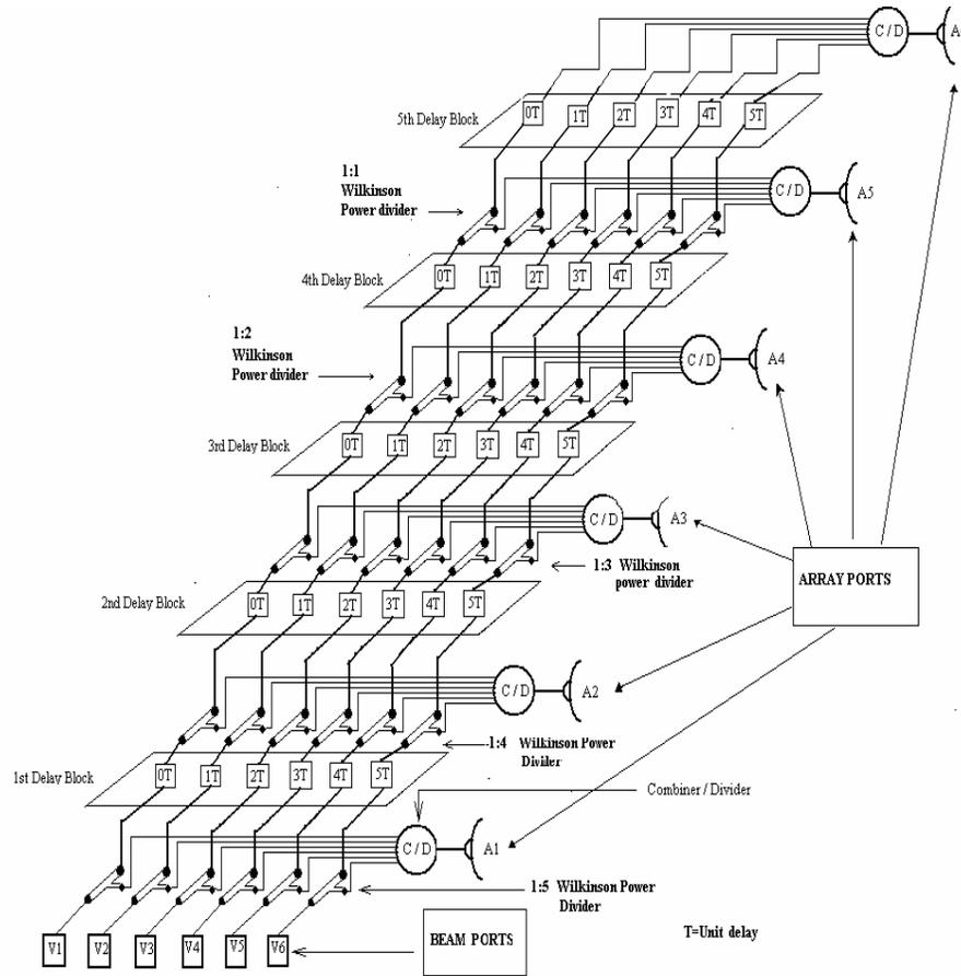
**Figure 2.** Schematic of multiple beam forming network using delay lines.
