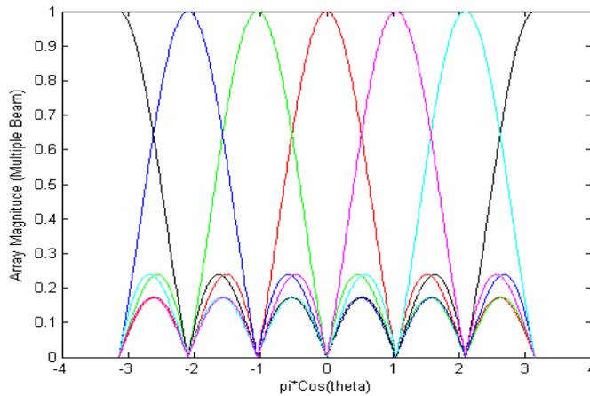
**Figure 3.** Array pattern for six individual sources.
