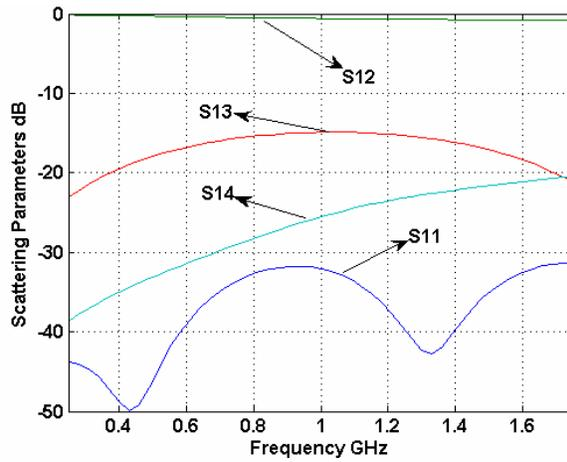
**Figure 8.** Simulated performance of the conventional coupler.
