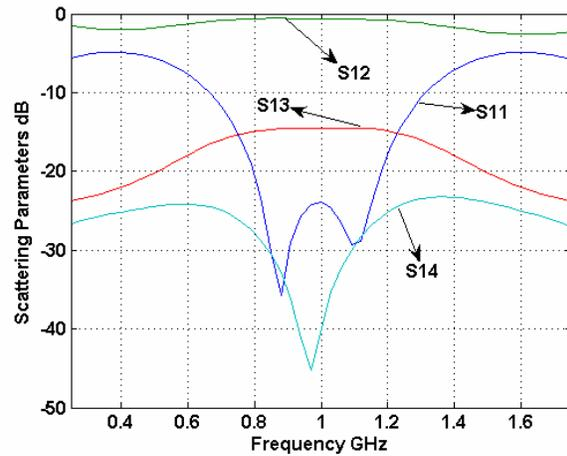
**Figure 9.** Simulated performance of the proposed coupler.
