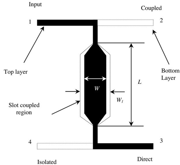
**Figure 2.** Layout of the microstrip slot-coupled directional coupler.
