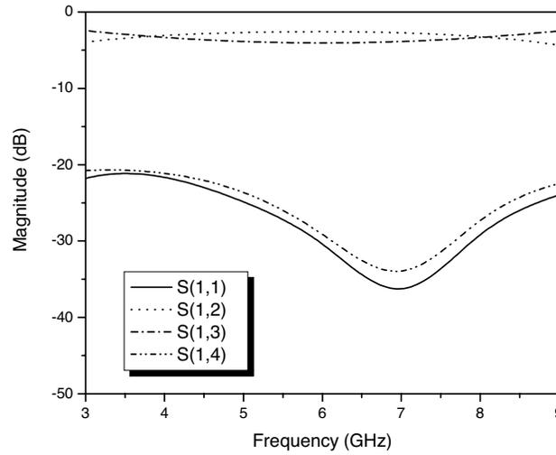
**Figure 3.** Simulated Scattering parameters of the directional coupler.
