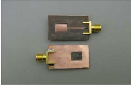
**Figure 6.** Photograph of the fabricated transition.
