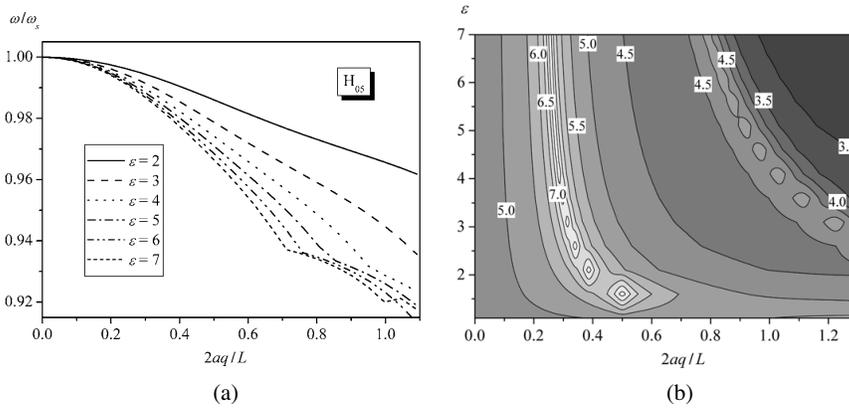
**Figure 4.** The resonant frequency shift (a) of the ORC  $H_{05}$ -mode and the radiation Q-factor (b) depending on the parameters of the dielectric test rod.
