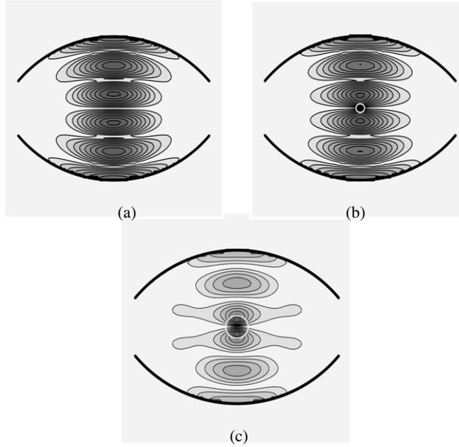
**Figure 6.** The resonance H-component field distribution across the ORC for the  $H_{05}$ -mode, the amplitude step  $0.1H_{\max}$ : (a) empty OR, (b)  $2aq/L = 0.3$ ,  $\varepsilon' = 6$ , and (c)  $2aq/L = 0.74$ ,  $\varepsilon' = 7$ .
