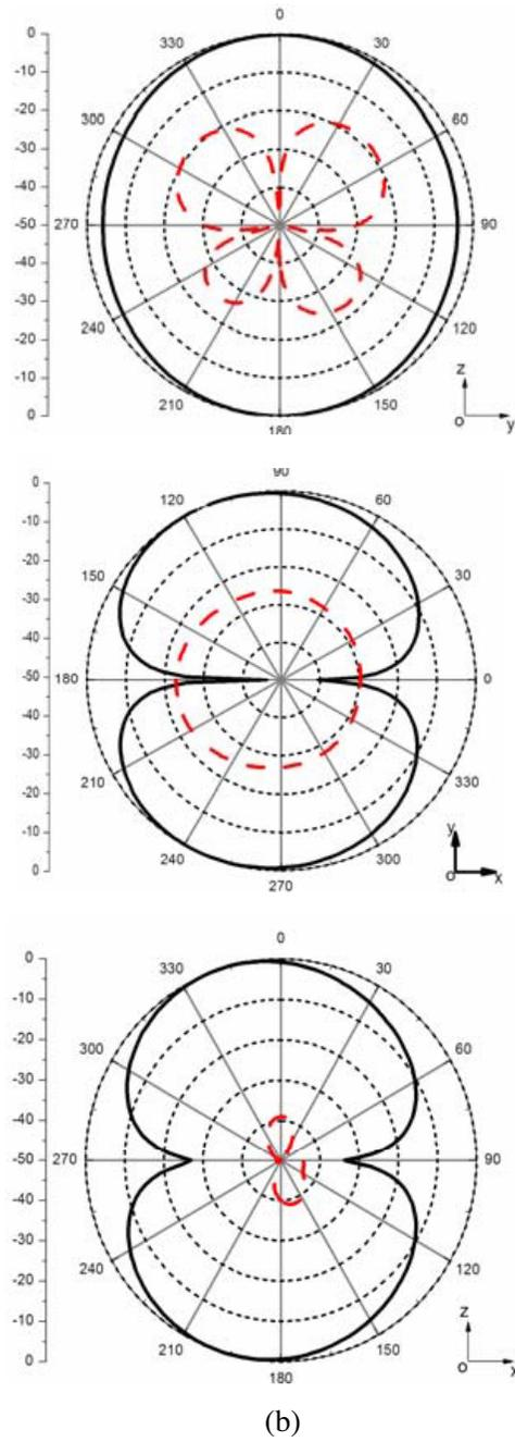
**Figure 6.** Radiation patterns of dual-band antenna with proposed CB-CPW at (a) 1.6 GHz and (b) 2.34 GHz.
