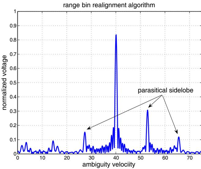
**Figure 6.** The integratoin output of range-bin realignment algorithm.
