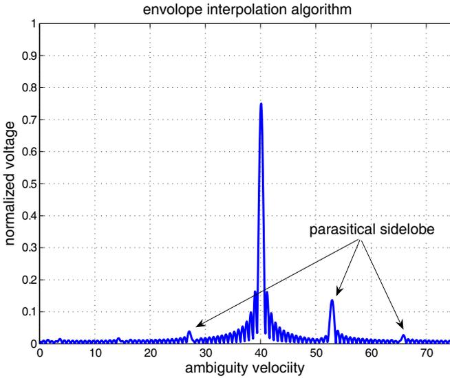
**Figure 7.** The integratoin outputs of envelope interpolation algorithm.
