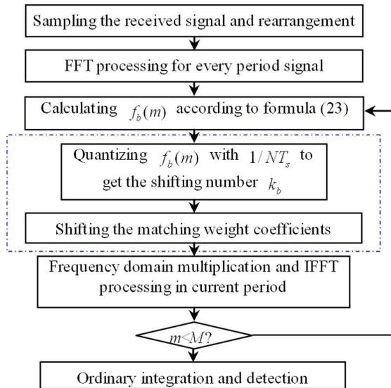
**Figure 2.** Long time coherent integration with migration compensation by shifting the matching weight coefficients.
