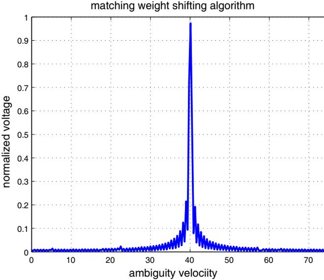
**Figure 9.** The integratoin output of the matching weight shifting algorithm (using 16 groups of weights).
