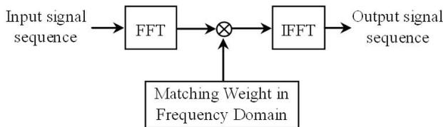
**Figure 1.** Digital match filtering performed in frequency domain.
