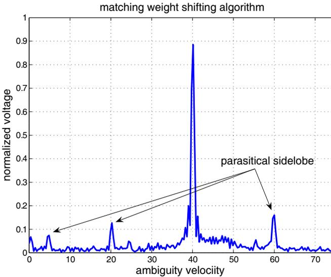
**Figure 8.** The integratoin output of the matching weight shifting algorithm (using single group of weight).
