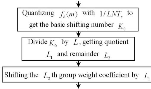
**Figure 3.** Choosing and shifting control of the matching weight coefficients when storing multi-groups of weight.
