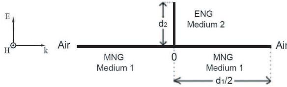
**Figure 1.** Scheme of the structure formed out of a finite MNG backbone and a single ENG side branch in the middle.
