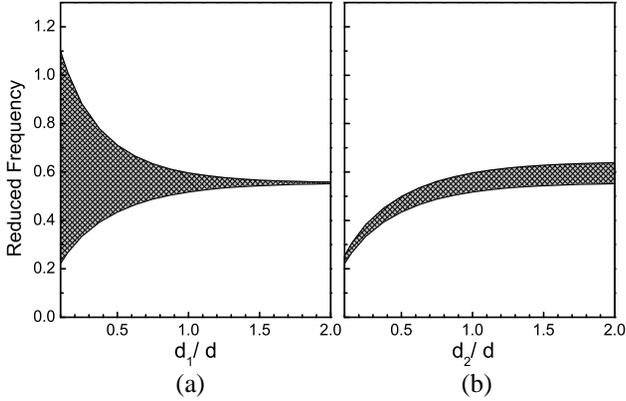
**Figure 6.** Variance of the band width with the distance between two neighboring side branches (a) and with the length of the side branches (b). The electromagnetic parameters are same as those for Fig. 5.
