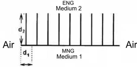
**Figure 4.** Scheme of the comb structure with periodic array of side branches.
