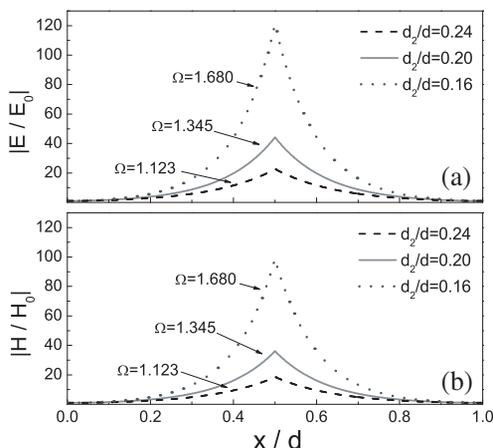
**Figure 3.** Spatial distributions of  $|E/E_0|$  (a) and  $|H/H_0|$  (b) at the frequencies of complete transmission for the structure with parameters  $\varepsilon_1 = 4$ ,  $\mu_1 = -6$ ,  $\varepsilon_2 = -6$ ,  $\mu_2 = 1$ ,  $d_1 = d$  and  $d_2/d = 0.24, 0.20, 0.16$ , and the corresponding reduced frequencies are 1.123, 1.345, 1.680, respectively.
