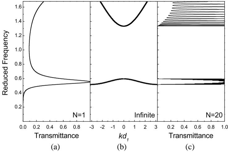
**Figure 5.** (a) Transmittance through a unit cell embedded in the air. (b) Band structure of an infinite comb structure. (c) Transmittance through a finite size comb structure with  $N = 20$  side branches.
