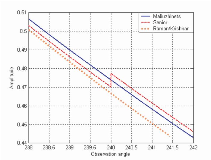
**Figure 4.** Comparison of the scattered waves at the shadow boundary.
