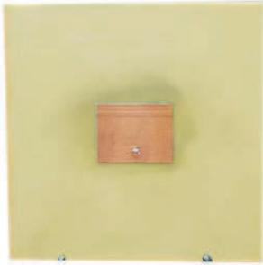
**Figure 12.** Single patch microstrip antenna.
