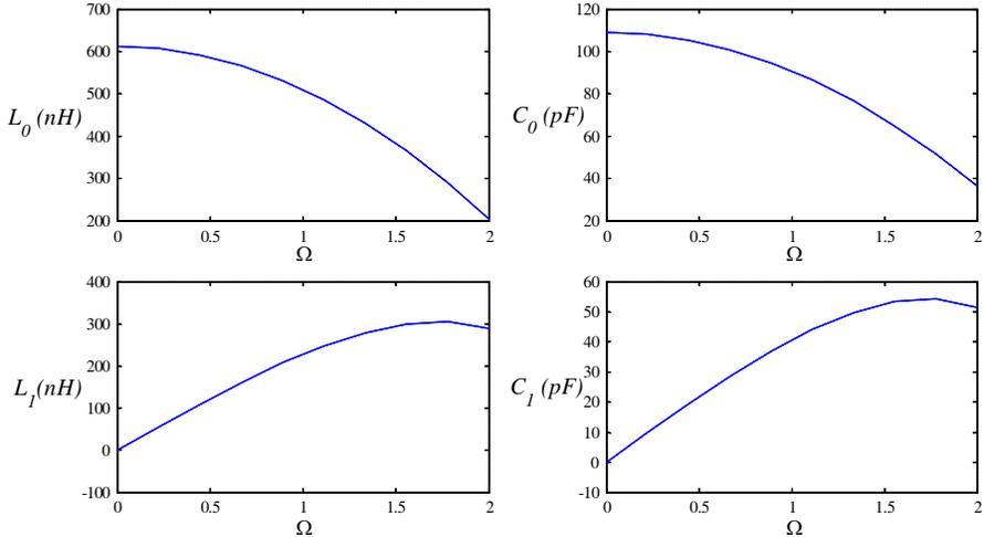
**Figure 5.** Elements of the equivalent circuit for pseudo-chiral stripline of Fig. 4 versus  $\Omega$ . Dimensions are:  $w = 2$  mm and  $h = 4$  mm and the parameters of the medium are:  $\varepsilon_t = 3$ ,  $\varepsilon_n = 2$ ,  $\mu_t = 2$ , and  $\mu_n = 1$ .
