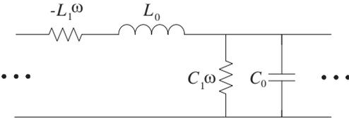
**Figure 3.** Equivalent circuit model for TEM mode propagation.
