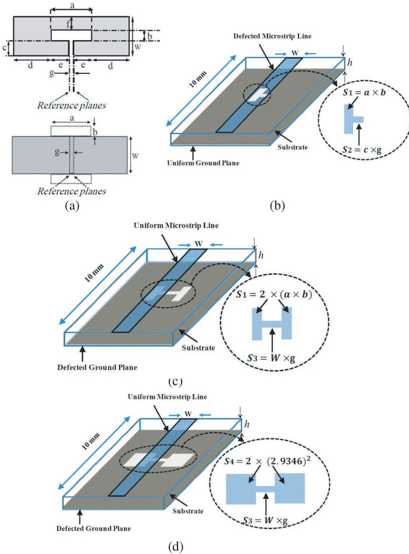
**Figure 1.** (a) Unit cell DMS and DGS parameters with  $a = 6.2$  mm,  $b = 0.5728$  mm,  $c = 1.3572$  mm,  $d = 1.9$  mm,  $e = 3$  mm,  $f = 0.4$  mm and  $g = 0.2$  mm, and (b), (c) and (d) 3D view of the DMS and DGS interconnections with the almost same resonant frequencies.
