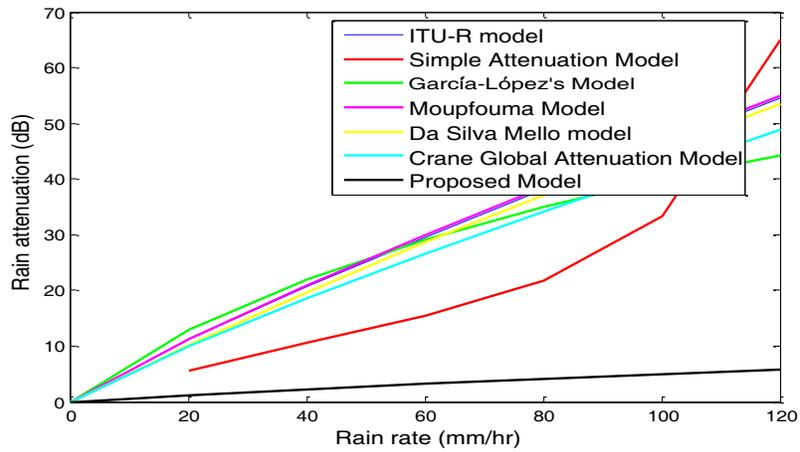
Figure 6. Comparison between suggested model and other existing models for distance 2 km.
