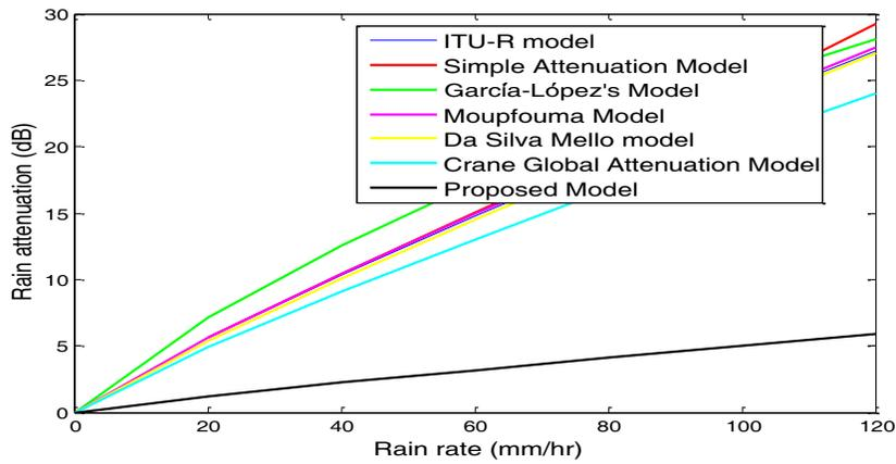
Figure 4. Comparison between suggested model and other existing models for 38 GHz.
