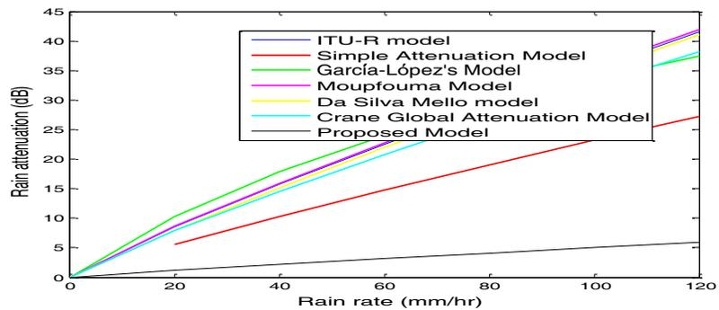
Figure 8. Comparison between suggested model and other existing models for 45° elevation angle.
