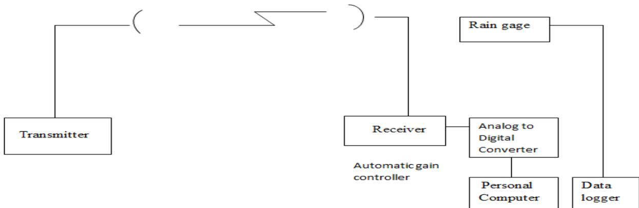
Figure 2. Experimental set up for data collection of rainfall.
