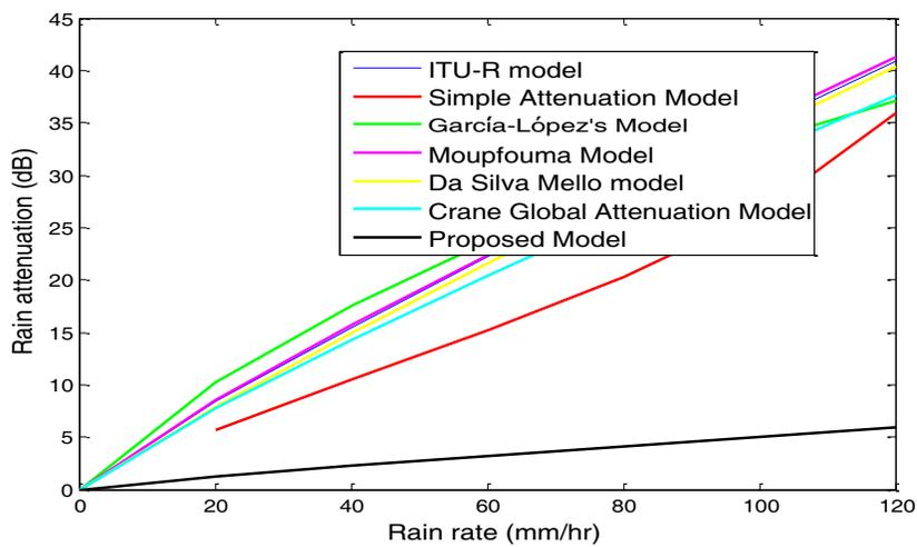
Figure 5. Comparison between suggested model and other existing models for distance 1.5 km.
