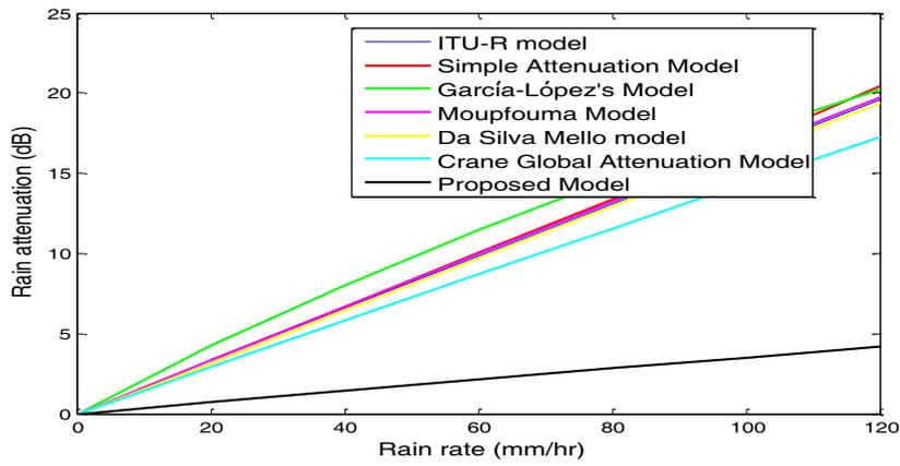
Figure 3. Comparison between suggested model and other existing models for 26 GHz.
