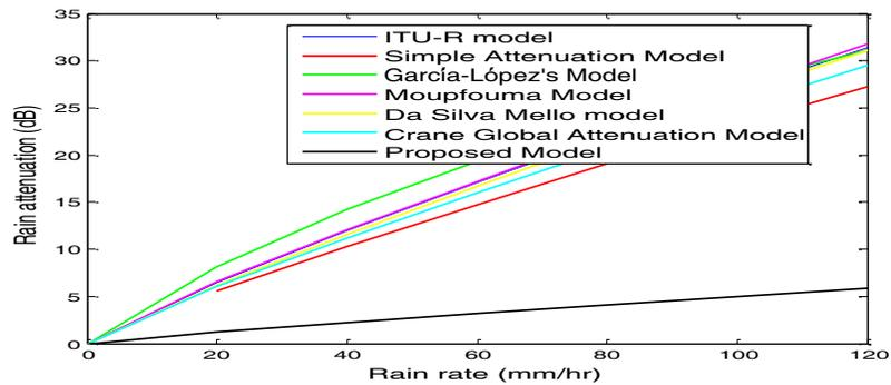
Figure 7. Comparison between suggested model and other existing models for 30° elevation angle.
