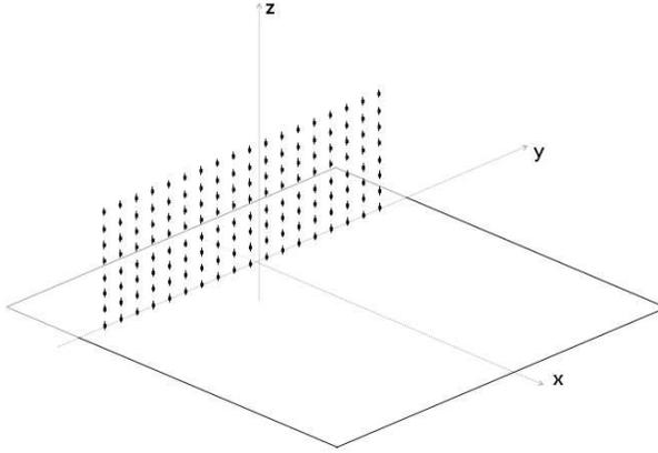
**Figure 5.** Geometry of the vertical current array. Each line is constituted by a number of vertical Hertzian dipoles in order to discretize the vertical current distribution.
