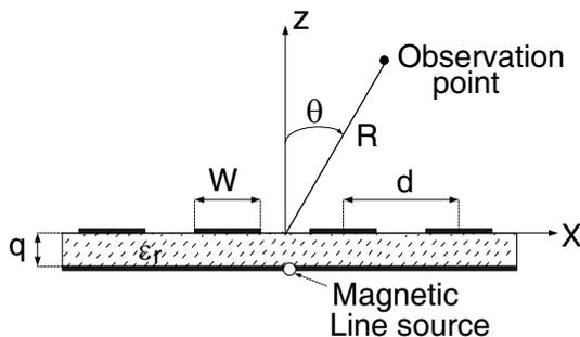
**Figure 1.** The geometry of a periodic structure excited by a magnetic line source in the  $y$  direction located at the ground plane (representing slot excitation). The structure consists of a metal strip grating over a grounded dielectric slab (GDS).
