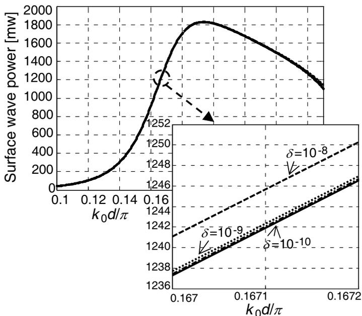
**Figure 2.** SW Power vs. frequency. Comparison between the proposed method and the numerical limit method for different values of  $\delta$  with pole location accuracy of  $10^{-15}$ . Legend: solid line-proposed method; dashed line-num. limit with  $\delta = 10^{-8}$ ; dotted line-num. limit with  $\delta = 10^{-9}$ ; dashed-dotted line-num. limit with  $\delta = 10^{-10}$ .
