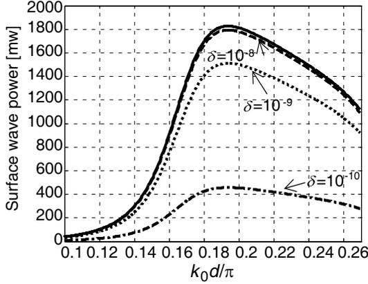
**Figure 3.** Re-calculation of the results of Fig. 2 with reduced pole location accuracy of  $10^{-10}$ . Comparison of the proposed method to the numerical limit method with different values of  $\delta$ . Legend: solid line-proposed method; dashed line-num. limit with  $\delta = 10^{-8}$ ; dotted line-num. limit with  $\delta = 10^{-9}$ ; dashed-dotted line-num. limit with  $\delta = 10^{-10}$ .
