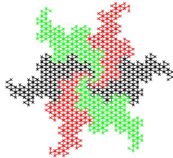
**Figure 5.** The 6-terdragon fractile array for the stage of growth  $P = 5$  whose elements are distributed uniformly along the 6-terdragon; each of which is represented by “x”. Note that the numbering scheme is not shown (From [1, 7]).
