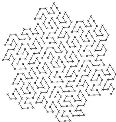
**Figure 2.** The Peano-Gosper fractal array for the stage of growth  $P = 3$  whose the first to the last elements are distributed uniformly along the Peano-Gosper curve (darkened curve) from the leftmost to the rightmost ends, respectively; each of which is represented by “x”. Note that the numbering scheme is not shown (From [1, 9]).
