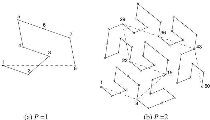
**Figure 1.** The Peano-Gosper fractal array for the first two stages of growth the first to the last whose elements are distributed uniformly along the Peano-Gosper curve (darkened curve) from the leftmost to the rightmost ends, respectively; each of which is represented by “x”. The dashed curve represents the Peano-Gosper curve represents the Peano-Gosper curve at the previous stage (From [1, 9]).
