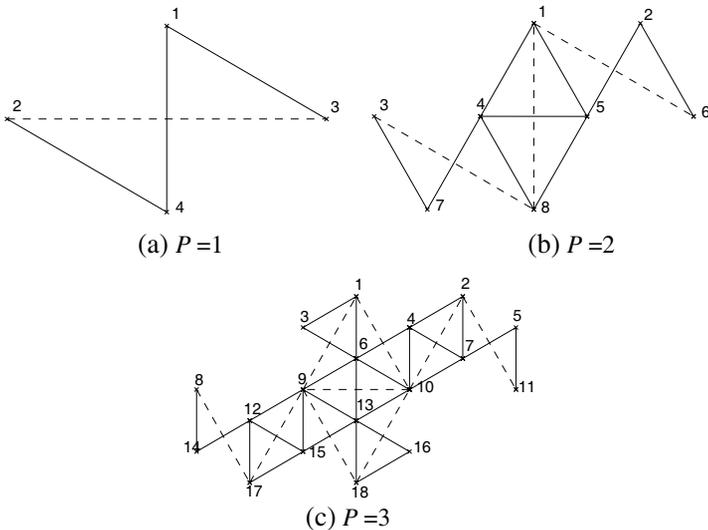
**Figure 3.** The terdragon fractile array for the first three stages of growth whose elements are distributed uniformly along the terdragon curve (darkened curve); each of which is represented by “x”. Elements are numbered from the farthest left to the farthest right and from the top to bottom. The dashed curve represents the terdragon curve at the previous stage (From [1, 7]).
