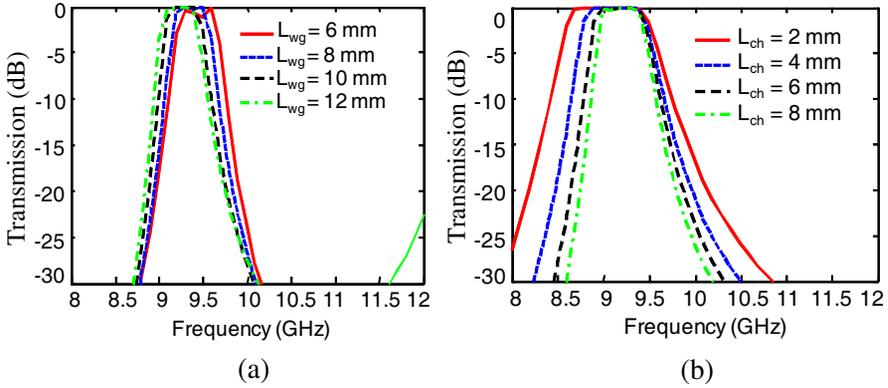
**Figure 4.** Transmission of the cascaded three-stage super-tunneling structure. (a) Maintain  $L_{ch} = 10$  mm to vary  $L_{wg}$  from 6 mm to 12 mm; (b) maintain  $L_{wg} = 12$  mm to vary  $L_{ch}$  from 2 mm to 8 mm.
