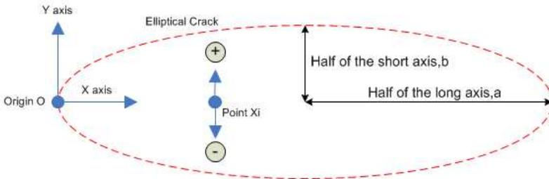
**Figure 1.** The elliptical crack and the oscillating directions of dipole in the crack.
