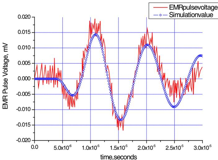
**Figure 3.** The simulation result for Rabinovitch’s compression granite experiment (Rabinovitch et al., 1998 [16]), the dashed line and the solid line are for experimental result and simulated result, respectively.
