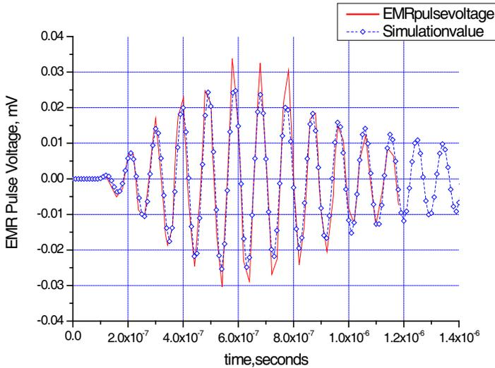
**Figure 4.** The simulation result for Rabinovitch's compression chalk experiment (Rabinovitch et al., 2000 [17]), the dashed line and the solid line are for experimental result and simulated result, respectively.
