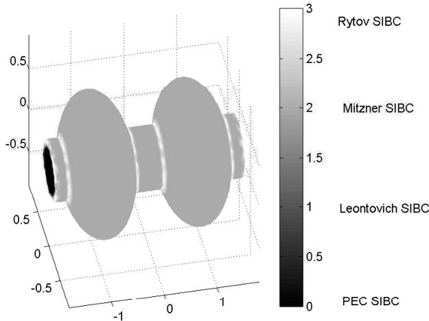
**Figure 2.** Piecewise surface impedance boundary conditions.
