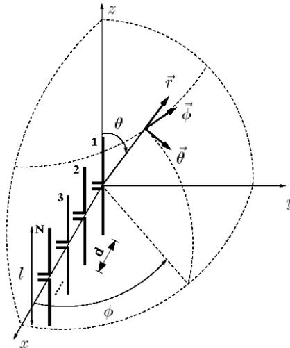
**Figure 1.** Geometry of linear array of parallel half-wave length dipole antennas.
