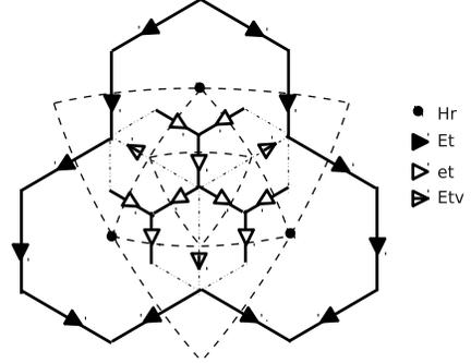
**Figure 4.** The possible subgrid technique for hexagonal grid-cell, virtual field quantities (Etv) are added to form completely FDTD algorithm.
