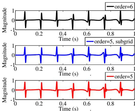
**Figure 5.** ELF wave propagation validation. A source is placed in a normal grid-cell and observed in the antipode of the sphere under different simulation conditions. Top: simulating using order 6 normal geodesic algorithm; middle: simulating using 5th order geodesic algorithm and subgrid technique; bottom: simulating using 5th order geodesic algorithm.
