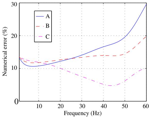
**Figure 8.** Comparison of numerical errors at different conditions: A) 4th order simulation; B) 4th order simulation with 1 subgrid (observation grid); C) 4th order simulation with 18 subgrids (including observation grid). The numerical errors are obtained by comparing these results to the 5th order simulation result.
