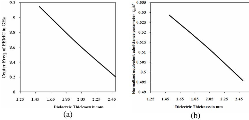
**Figure 9.** The effect of the dielectric thickness. (a) Center frequency of PEMC boundary as a function of the dielectric thickness. The tilting angles between the patches  $\theta = 45^\circ$ . (b) Normalized equivalent admittance parameter of PEMC boundary as a function of the dielectric thickness. The tilting angles between the patches  $\theta = 45^\circ$ .
