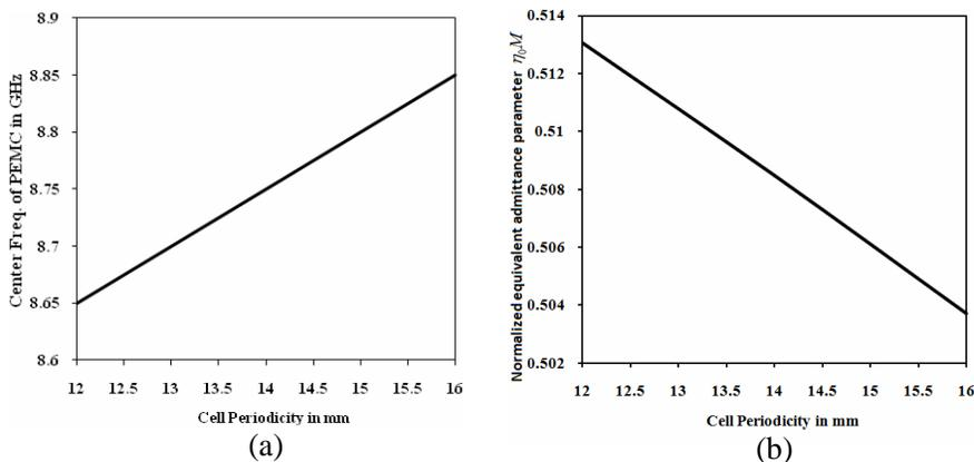
**Figure 8.** The effect of the cell periodicity. (a) Center frequency of PEMC boundary as a function of the cell periodicity. The tilting angles between the patches  $\theta = 45^\circ$ . (b) Normalized equivalent admittance parameter of PEMC boundary as a function of the cell periodicity. The tilting angles between the patches  $\theta = 45^\circ$ .
