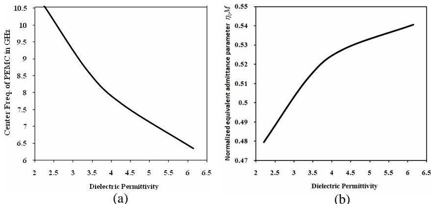
**Figure 10.** The effect of the dielectric permittivity. (a) Center frequency of PEMC boundary as a function of the dielectric permittivity. The tilting angles between the patches  $\theta = 45^\circ$ . (b) Normalized equivalent admittance parameter of PEMC boundary as a function of the dielectric permittivity. The tilting angles between the patches  $\theta = 45^\circ$ .
