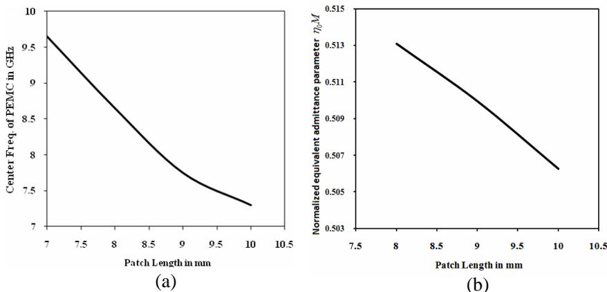
**Figure 7.** The effect of the patch length. (a) Center frequency of PEMC boundary as a function of the length of the patch. The tilting angles between the patches  $\theta = 45^\circ$ . (b) Normalized equivalent admittance parameter of PEMC boundary as a function of the length of the patch. The tilting angles between the patches  $\theta = 45^\circ$ .
