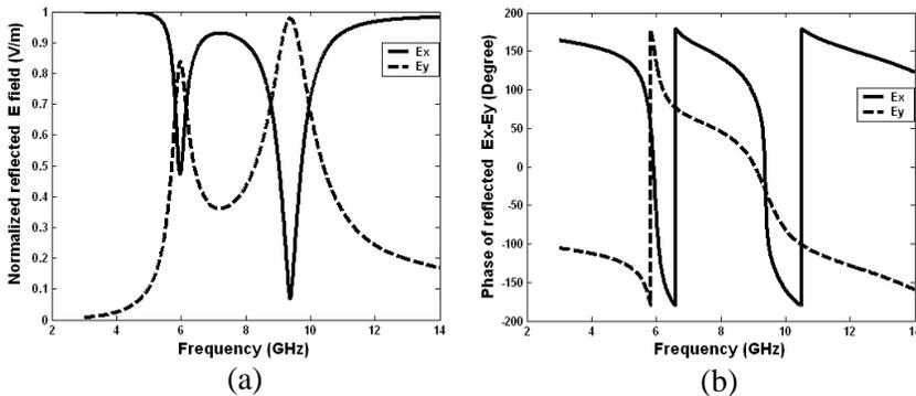
**Figure 3.** Reflection coefficients of co-polarized and cross-polarized field components. The tilting angles between the patches  $\theta = 90^\circ$ . (a) Amplitudes of reflection coefficients. (b) Phase of reflected coefficients.
