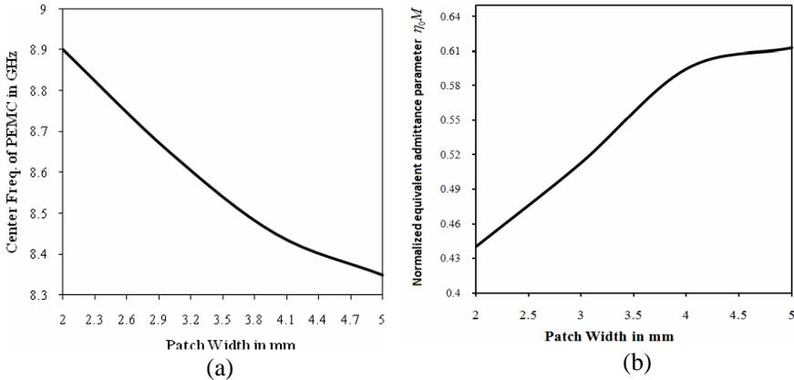
**Figure 6.** The effect of the patch width. (a) Center frequency of PEMC boundary as a function of the patch width. The tilting angles between the patches  $\theta = 45^\circ$ . (b) Normalized equivalent admittance parameter of PEMC boundary as a function of the patch width. The tilting angles between the patches  $\theta = 45^\circ$ .
