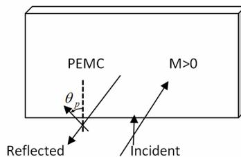
**Figure 1.** The polarization of reflected wave due to a PEMC boundary is rotated by an angle  $\theta_p$  with respect to the polarization of the incident wave [6].
