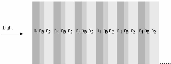
**Figure 2.** Schematic of 1D ternary PBG structure.
