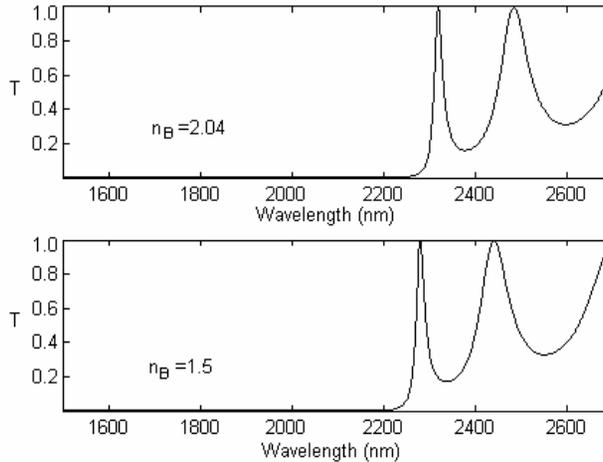
**Figure 3.** Transmission spectra for 1D ternary PBG structure with  $n_1 = 3.3$ ,  $n_B = 2.04$  and  $1.5$ ,  $n_2 = 1.46$ ,  $d_1 = 117$  nm,  $d_B = 40$  nm,  $d_2 = 265$  nm and  $N = 10$  at  $0^\circ$  angle of incidence of light.
