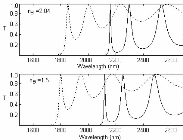
**Figure 5.** Transmission spectra for 1D ternary PBG structure with  $n_1 = 3.3$ ,  $n_B = 2.04$  and  $1.5$ ,  $n_2 = 1.46$ ,  $d_1 = 117$  nm,  $d_B = 40$  nm,  $d_2 = 265$  nm and  $N = 10$  at  $45^\circ$  angle of incidence of light.
