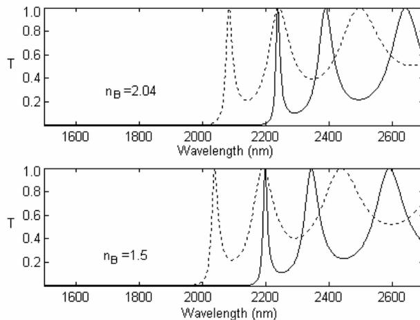
**Figure 4.** Transmission spectra for 1D ternary PBG structure with  $n_1 = 3.3$ ,  $n_B = 2.04$  and  $1.5$ ,  $n_2 = 1.46$ ,  $d_1 = 117$  nm,  $d_B = 40$  nm,  $d_2 = 265$  nm and  $N = 10$  at  $30^\circ$  angle of incidence of light.
