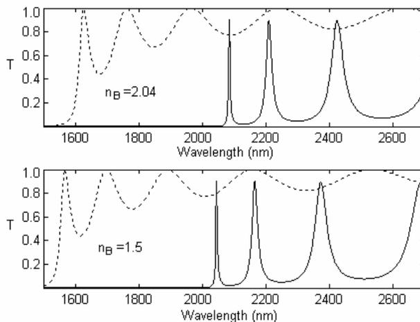
**Figure 6.** Transmission spectra for 1D ternary PBG structure with  $n_1 = 3.3$ ,  $n_B = 2.04$  and  $1.5$ ,  $n_2 = 1.46$ ,  $d_1 = 117$  nm,  $d_B = 40$  nm,  $d_2 = 265$  nm and  $N = 10$  at  $60^\circ$  angle of incidence of light.
