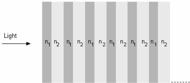
**Figure 1.** Schematic of 1D binary PBG structure.
