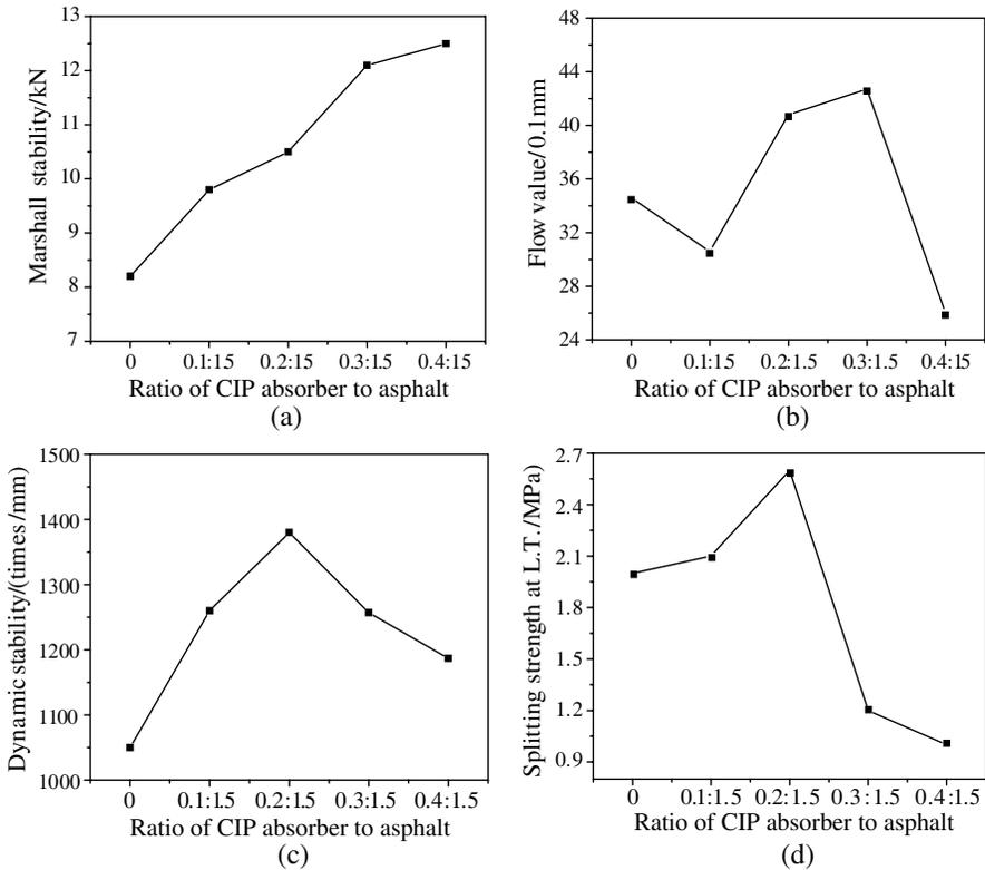
**Figure 5.** Properties of the asphalt mixes. (a) Marshall stability, (b) flow value, (c) dynamic stability, (d) splitting strength at low temperature.
