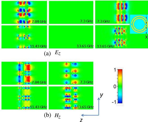
**Figure 4.** The simulated electric (a) and magnetic (b) fields distributions for the four stacked SRRs metasurfaces at the corresponding resonances, along the  $yz$ -middle-cutting plane, for vertical (left column) and horizontal (central column) polarizations, and along the  $x$  position of the  $yz$ -cutting plane for horizontal polarization (right column).
