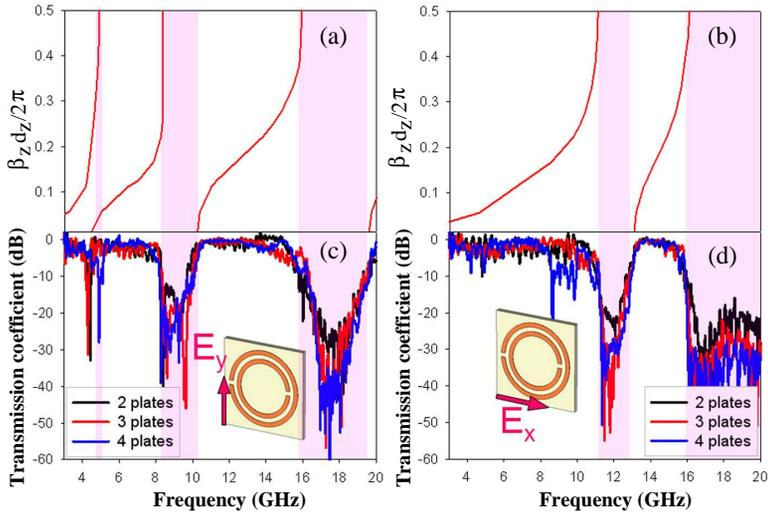
**Figure 2.** Simulated dispersion diagram for SRRs in axial configuration, vertical (a) and horizontal (b) polarization. Measurement of the transmission coefficient as a function of different number of stacked metasurfaces for vertical (c) and horizontal (d) polarizations. Insets: unit cell along with incident electric field.
