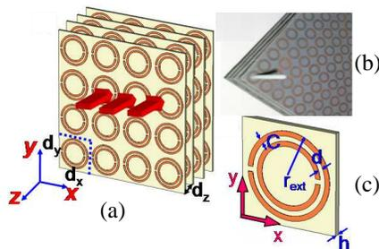
**Figure 1.** Schematic of stacked SRR (a), fabricated prototype (b) and unit cell (c).
