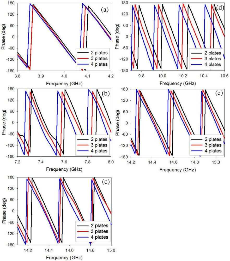
**Figure 5.** Phase response corresponding to the measured transmission coefficient for vertical (a) and horizontal (b) polarization, respectively.
