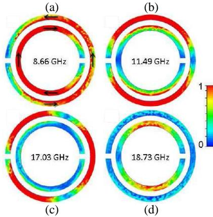
**Figure 3.** The current density distribution for vertical (a), (b) and horizontal (c), (d) polarisation, respectively, at each correspondence frequency.
