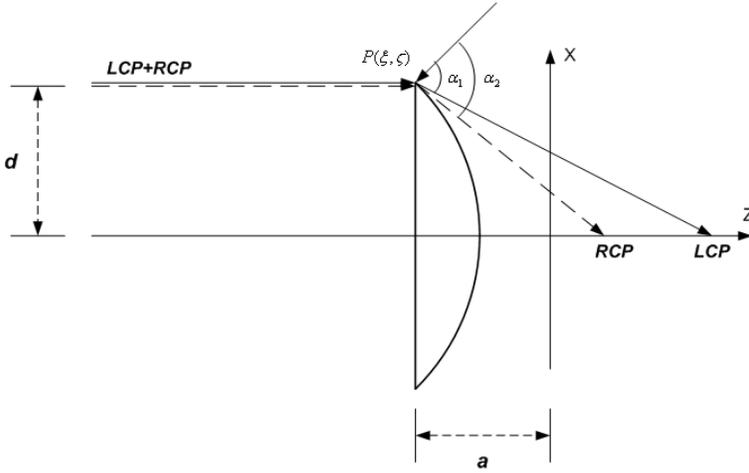
**Figure 5.** Hyperbolic lens placed in chiral medium.
