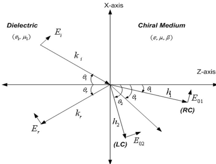
**Figure 3.** The incident, reflected and transmitted waves at an oblique incidence at dielectric-chiral interface [8].
