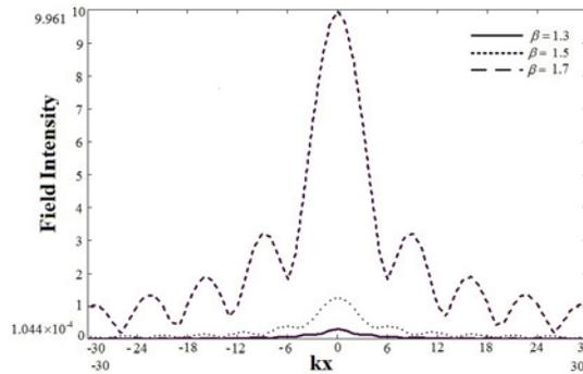
**Figure 9.** Field intensity of LCP wave for  $\beta = 1.3, 1.5, 1.7$ .
