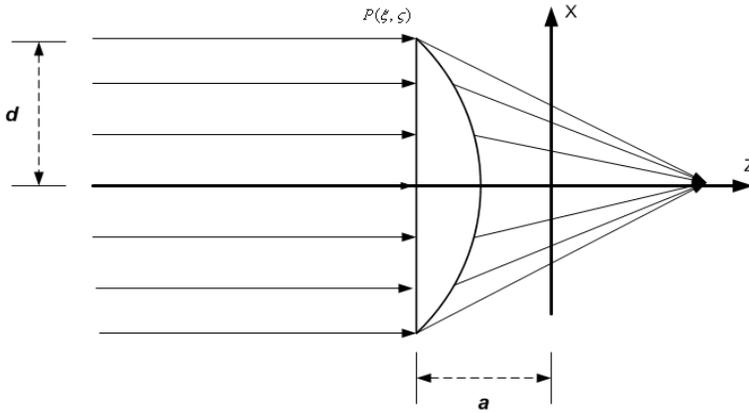
**Figure 4.** Fields and parameters of a hyperbolic lens.
