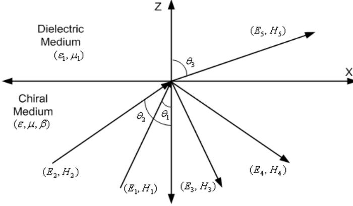
**Figure 2.** Waves traveling from chiral to dielectric medium [7].
