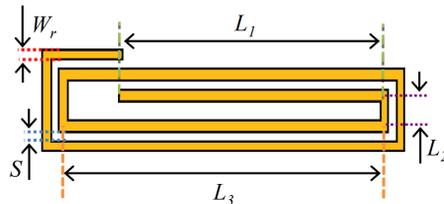
**Figure 1.** Particle structure with  $N = 2$  turns,  $W_r = 200 \mu\text{m}$ ,  $S = 200 \mu\text{m}$ ,  $L_1 = 6500 \mu\text{m}$ ,  $L_2 = 600 \mu\text{m}$  and  $L_3 = 8000 \mu\text{m}$ .
