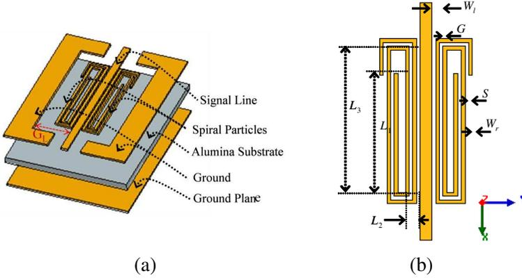
**Figure 3.** Structure of the proposed micro-resonator. (a) With the different stages. (b) Top view with the different geometrical parameters.
