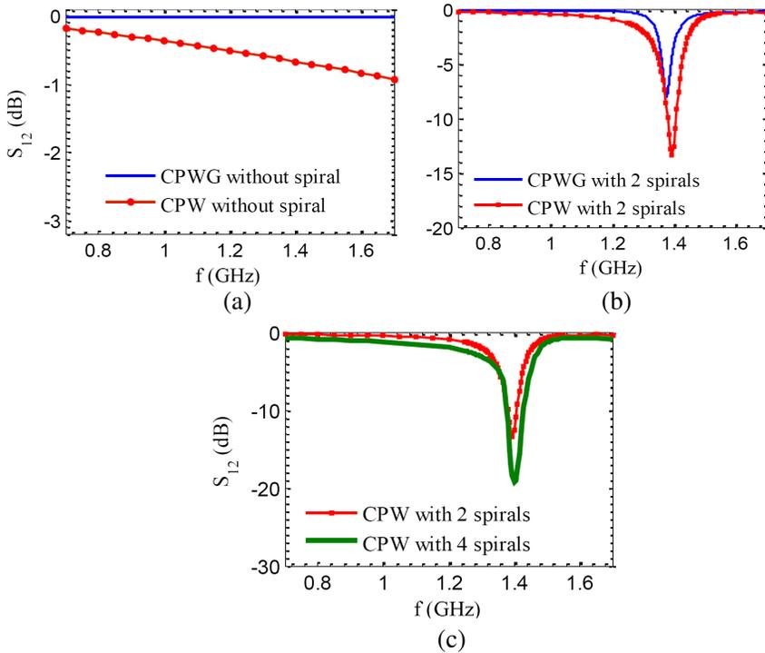
**Figure 5.** Simulated transmission coefficient of the micro-resonator. With  $N = 2$  turns,  $W_r = 635 \mu\text{m}$ ,  $W_l = 635 \mu\text{m}$ ,  $G_l = 1300 \mu\text{m}$ ,  $G = 200 \mu\text{m}$ ,  $S = 200 \mu\text{m}$ ,  $L_1 = 6500 \mu\text{m}$ ,  $L_2 = 600 \mu\text{m}$ ,  $L_3 = 8000 \mu\text{m}$ . (a) CPWG and CPW without spiral. (b) CPWG and CPW with 2 spirals. (c) CPW with 2 and 4 spirals.
