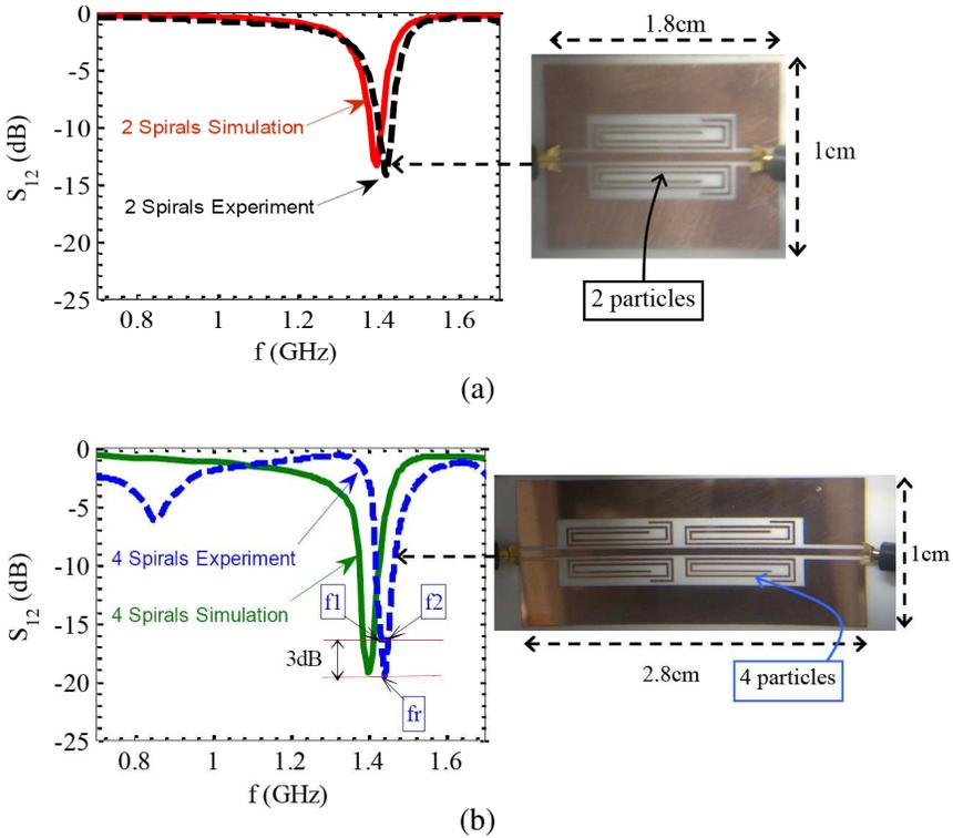
**Figure 6.** Experimental result of the insertion loss  $S_{12}$  (dB) for 2 and 4 particles. Such as:  $N = 2$  turns,  $W_r = 200 \mu\text{m}$ ,  $W_l = 635 \mu\text{m}$ ,  $G_l = 1300 \mu\text{m}$ ,  $G = 200 \mu\text{m}$ ,  $S = 200 \mu\text{m}$ ,  $L_1 = 6500 \mu\text{m}$ ,  $L_2 = 600 \mu\text{m}$ ,  $L_3 = 8000 \mu\text{m}$ . (a) Two particles placed on both sides of the transmission line. (b) Four particles placed on both sides of the transmission line.
